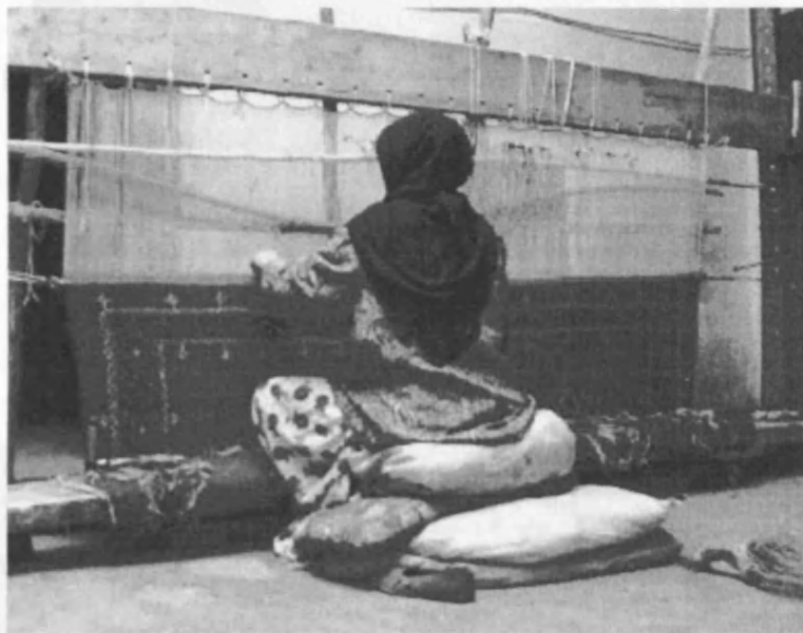
Figure 28 Last stage before cutting the carpet. The weaver is sitting high up, thanks to several cushions, her knees are situated above the beam and against the weaving, her arms are at breast level.
