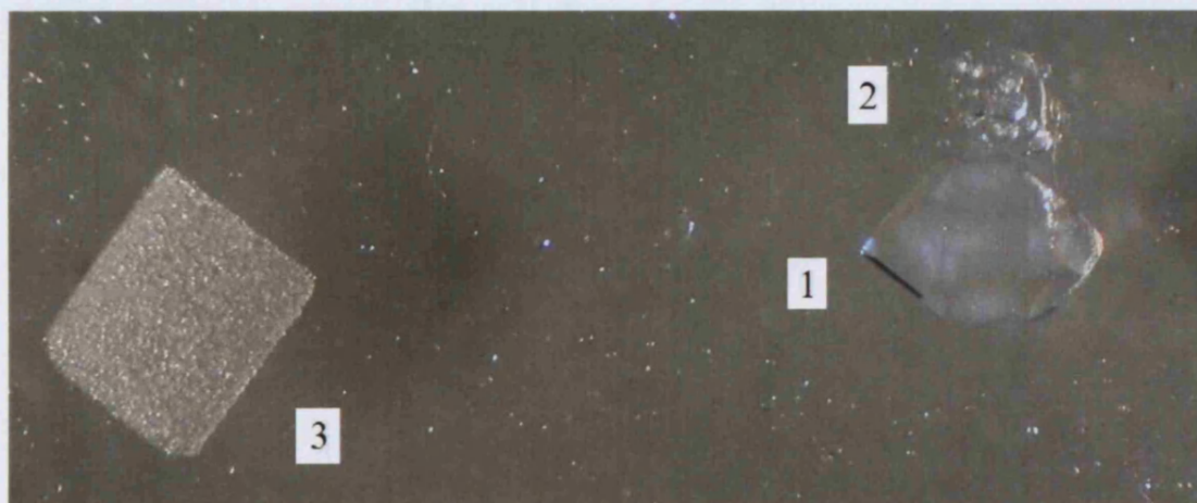
Figure 4.11. Photograph of the in situ phase change from form 2 to form 1. 1: form 1 crystal; 2: form 2 plate covered in form 1 blocks; 3: form 2 block early stage of phase transformation
