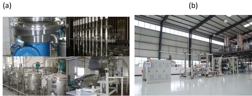
Figure 11 – Examples of equipment for spray drying for milk and whey powders (a), and of extrusion of cereals and pulses blends (b).
