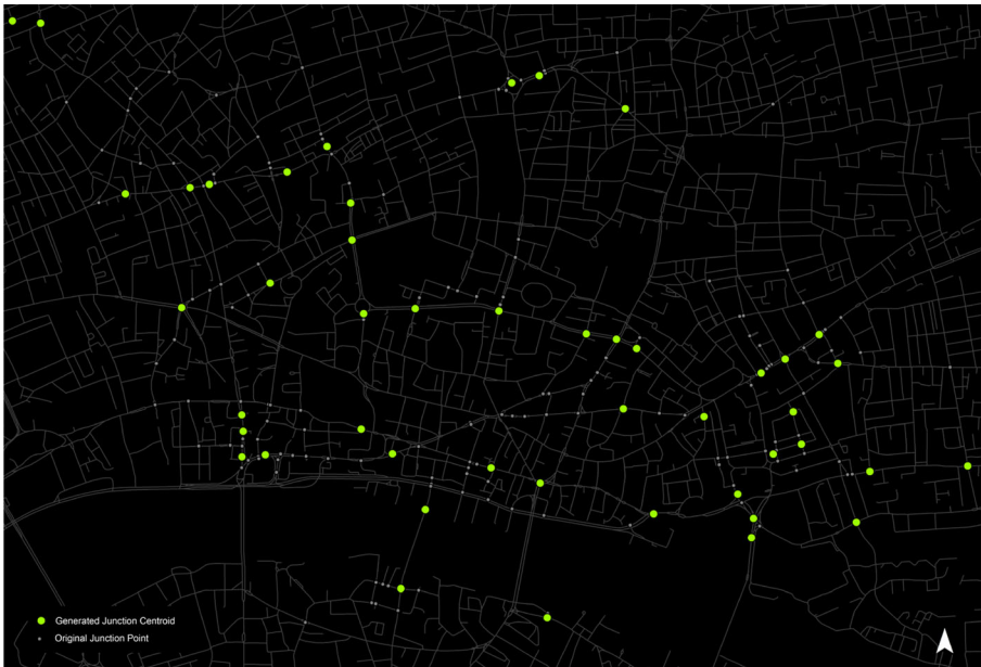
Fig. 2 Example of spatially clustered nodes (shown in green) formed from junction nodes (indicated in grey)
