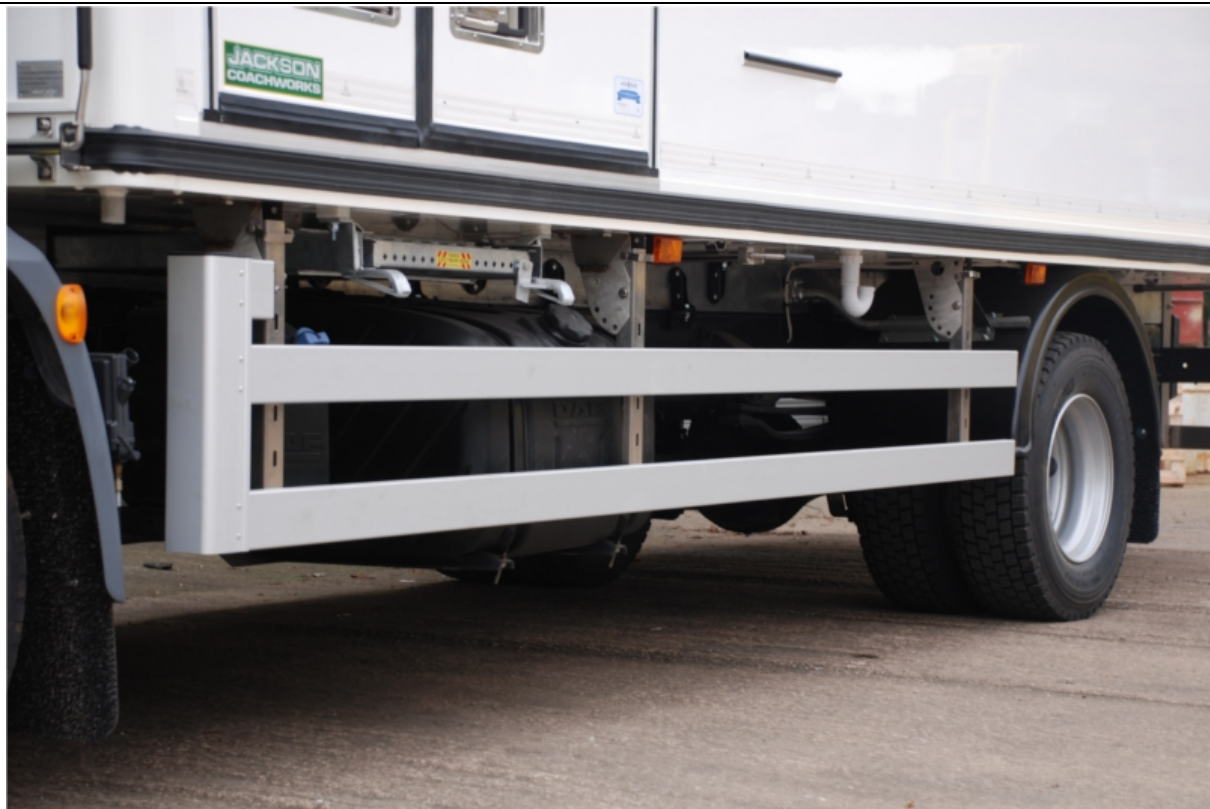
Figure 40: Basic side guard fitment compliant with current regulations
