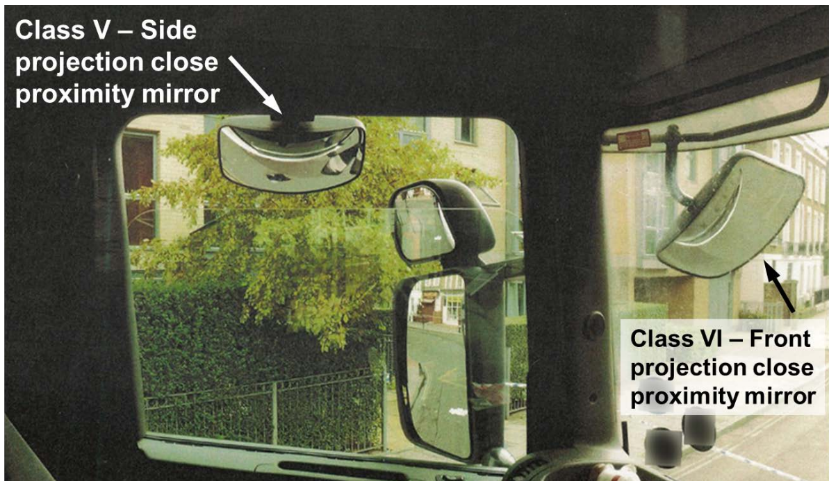
Figure 31: HGV mirrors – view from cab (Delmonte et al 2013)
