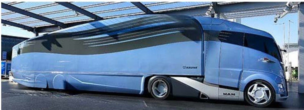
Figure 39: Concept truck design with extended side guards (MAN)
