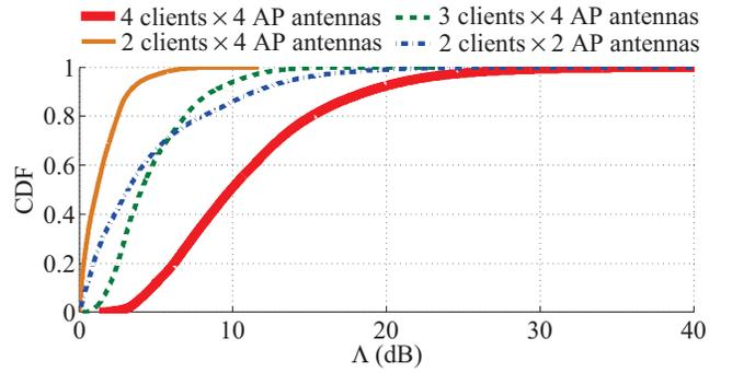
**Figure 10:** Cumulative distribution across testbed links and OFDM subcarriers of  $\Lambda$ , the SNR ratio degradation that the most-degraded user experiences for each particular link.
