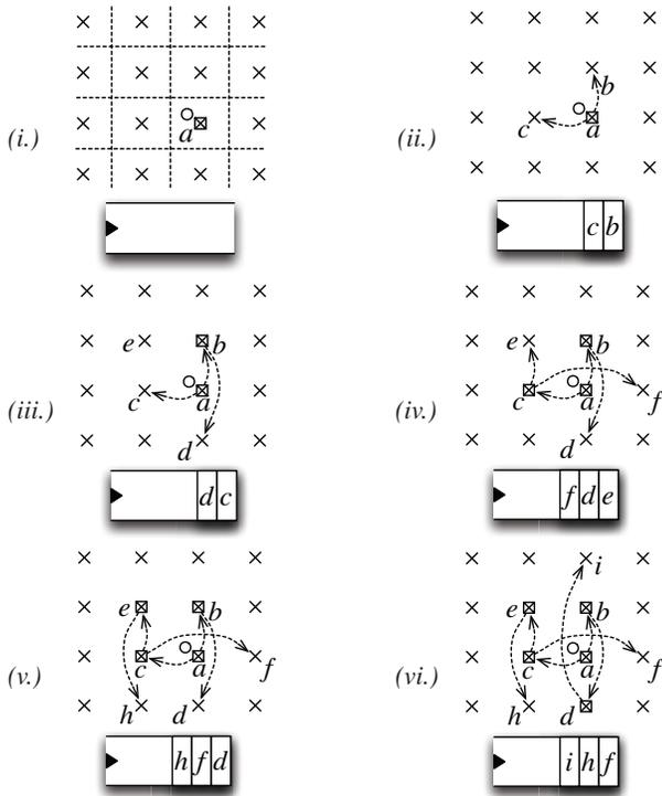
**Figure 6:** Geosphere’s two-dimensional zigzag enumeration in the 16-QAM constellation. We denote constellation points  $\times$ , label points whose partial Euclidean distances have been computed, and denote points that have been explored  $\boxtimes$ .
