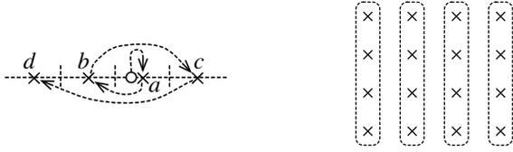
**Figure 4:** *Left:* The zigzag technique in a one-dimensional (PAM) constellation visits constellation points ( $\times$ ) in increasing distance from the received symbol ( $\circ$ ). *Right:* Dividing a 16-QAM constellation into four 4-PAM subconstellations.
