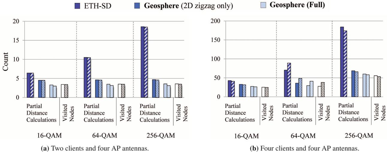
**Figure 15:** Simulation-based complexity comparison between ETH-SD and Geosphere. *Solid bars:* Simulated Rayleigh channel; *striped bars:* empirically measured channel. N.B.: each of the above sphere decoders visit the same number of nodes.
