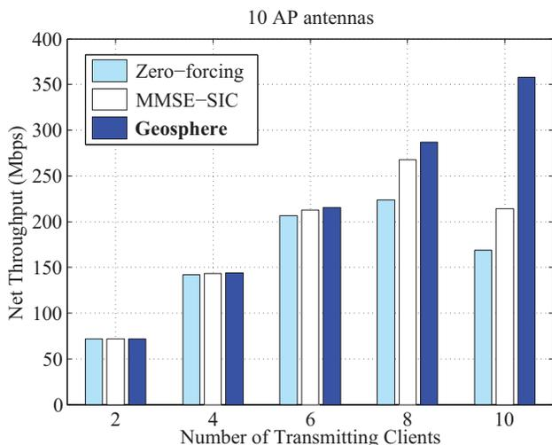
**Figure 13:** Simulation-based throughput comparison between zero-forcing MIMO, MMSE-SIC and Geosphere for different numbers of users accessing a ten-antenna AP at the same time over a Rayleigh fading channel.
