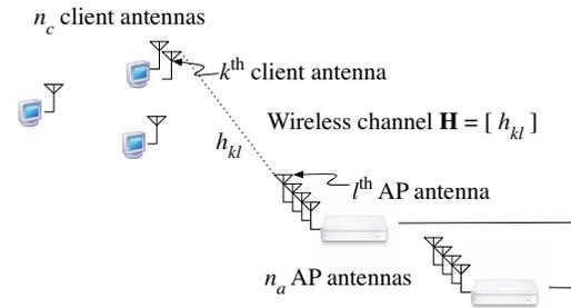
**Figure 1:** A MIMO wireless LAN with  $n_c$  client antennas and  $n_a$  AP antennas. Different clients and APs may transmit simultaneously, forming a MIMO system described by the channel matrix  $\mathbf{H}$ , whose entries characterize the wireless channel between a client’s antenna and an AP’s antenna.
