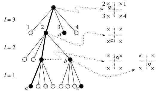
**Figure 3:** The sphere decoder operating on  $n_c = 3$  transmit antennas, each sending a QPSK ( $|\mathcal{O}| = 4$ ) symbol. Constellation points (denoted  $\times$ ) and corresponding branches of the tree are numbered at the uppermost level ( $l = 3$ ), and the received signal is denoted  $o$ . Visited nodes are colored black.
