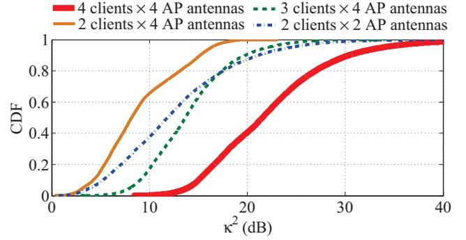
**Figure 9:** Cumulative distribution across testbed links, OFDM subcarriers, and spatial streams of  $\kappa^2$  (decibels), the power of the MIMO channel condition number. Higher values of  $\kappa^2$  indicate worse channel conditioning.
