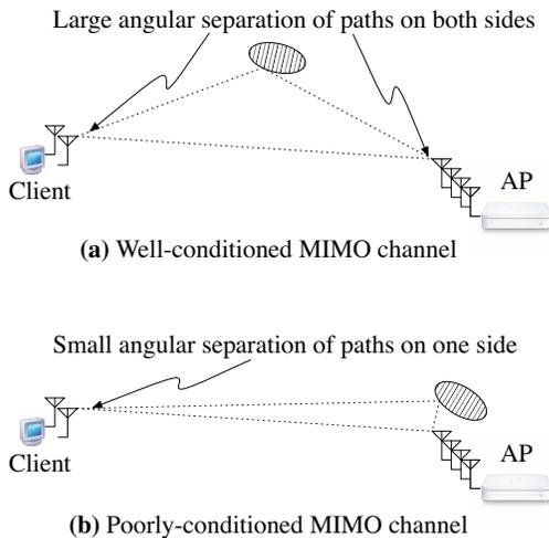
**Figure 2:** When reflectors are located solely in the vicinity of one of the endpoints of a MIMO link, the result is a very small angular separation of the energy arriving at the other end, and a poorly-conditioned channel matrix  $\mathbf{H}$ .
