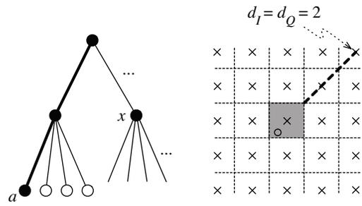
**Figure 7:** Geometrically lower-bounding the distance between received symbol  $\circ$  and another constellation point at horizontal ( $d_l$ ) and vertical ( $d_Q$ ) offset two from the closest constellation point. Constellation points are spaced two units apart.
