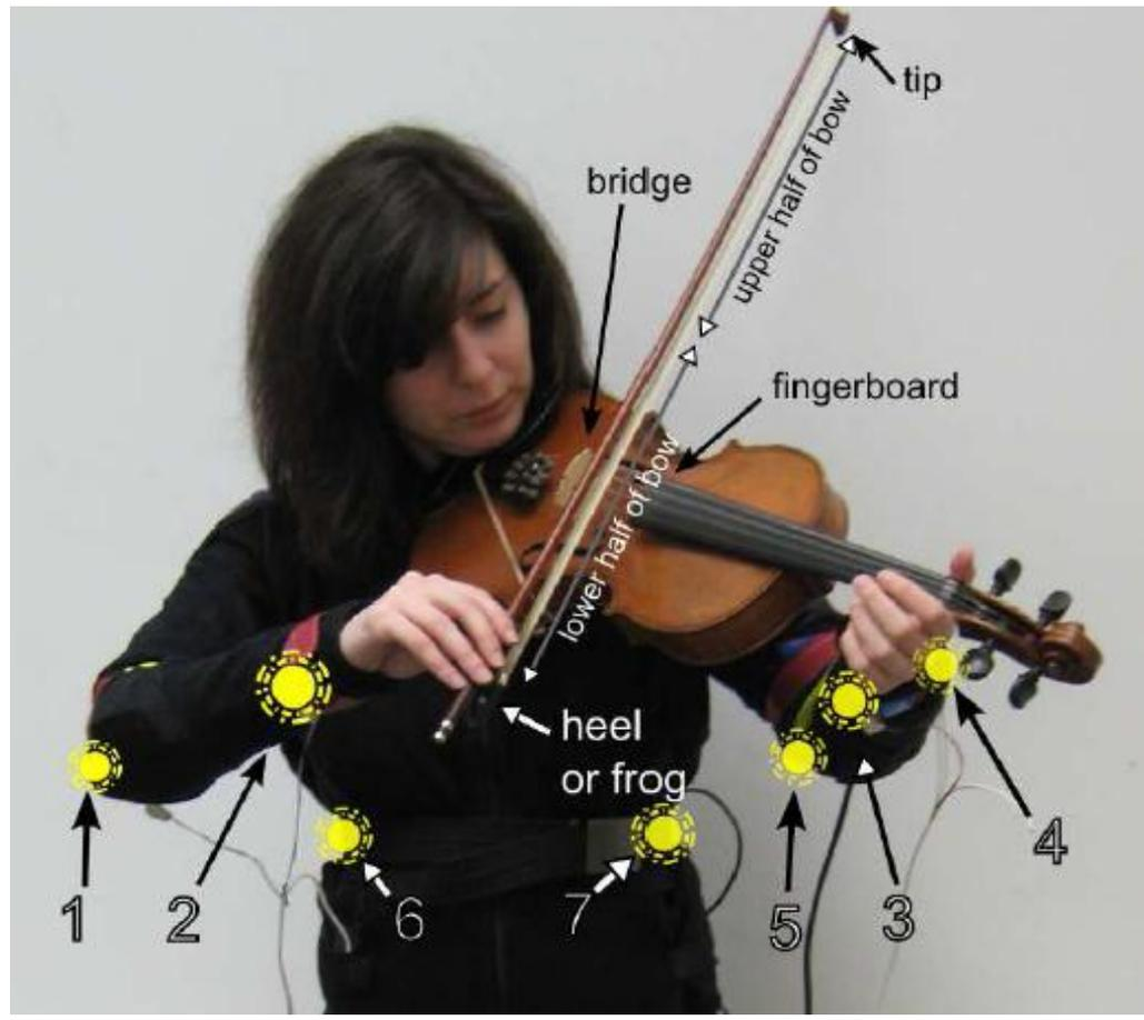
Figure A-9: Second prototype (1 move bow hand forward, 2 move bow hand back, 3 move violin left, 4 move violin right, 5, 6, 7 lift violin)
