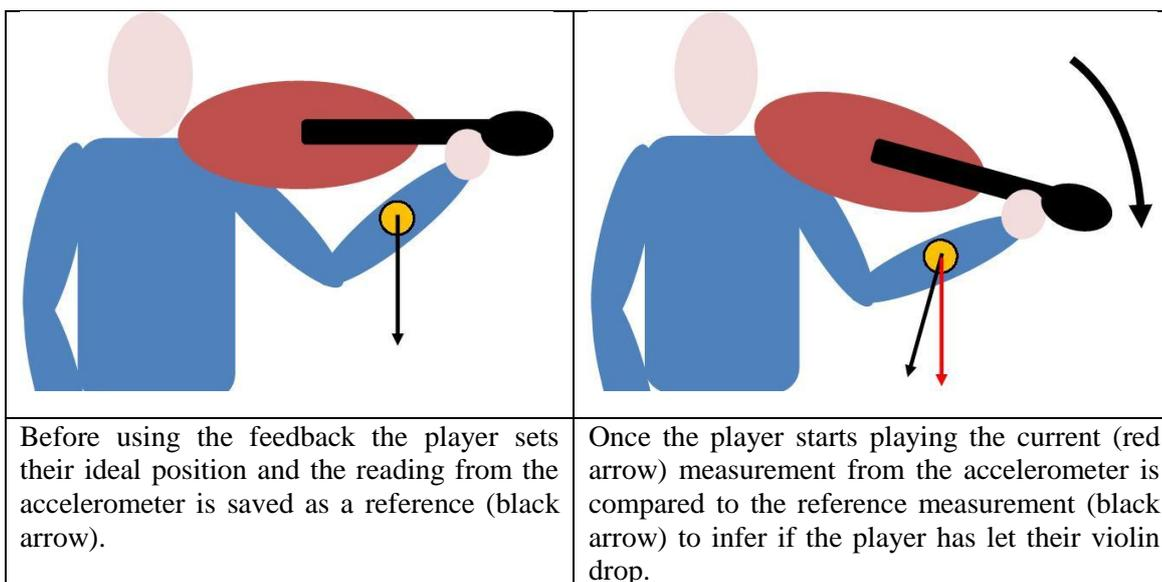
Figure 7-2: Diagram of how angle of arm can be measured using an accelerometer
