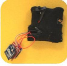
A vibrator is built in to a sweat band positioned on the right wrist and buzzes inform the player when they have used a 'good' amount of bow (full length in this study).
