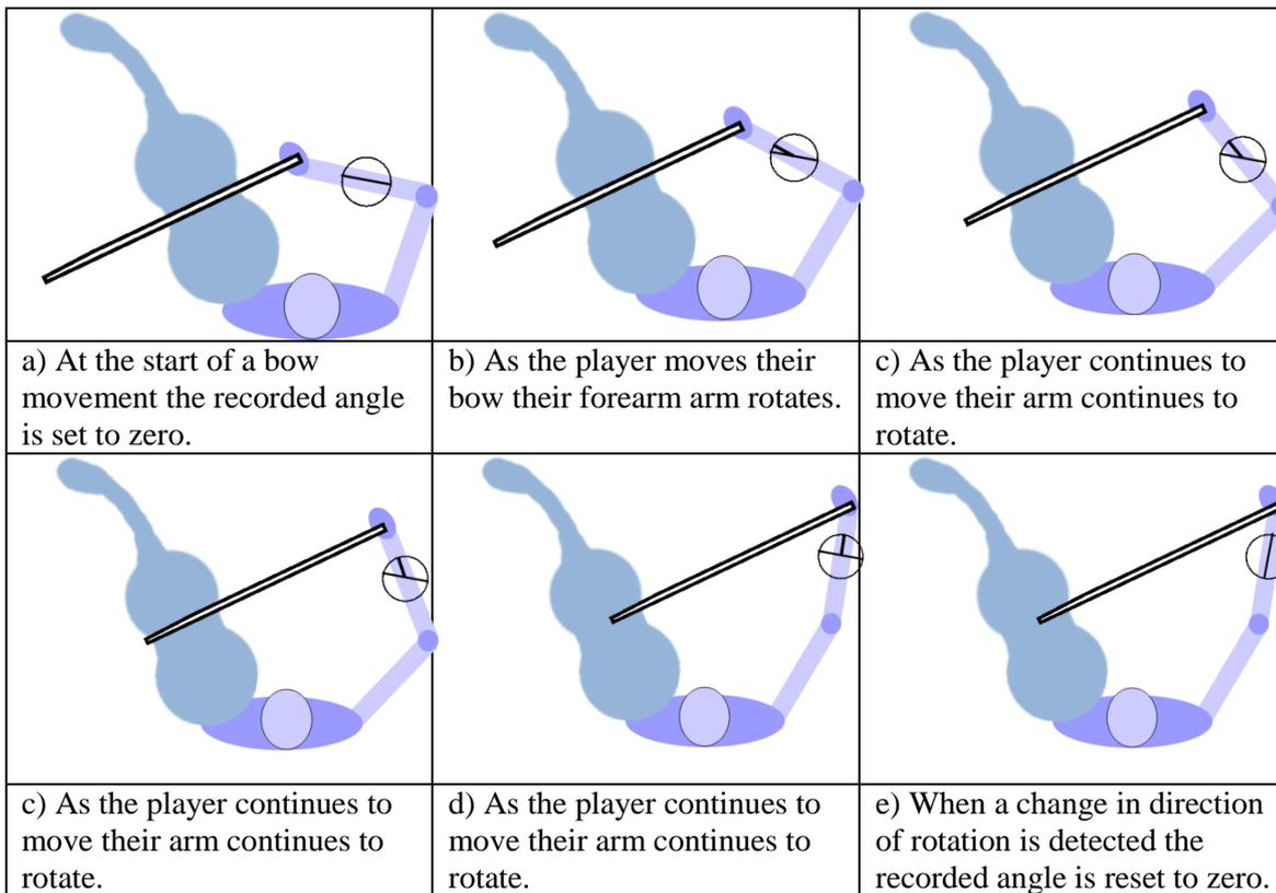
Figure 5-2: How the angle of the player's arm relates to the length of bow used
