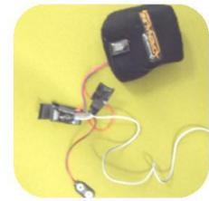
This sweat-band that is worn on the lower arm away from the wrist. It is designed to infer the length of bow the player uses by measuring the angle which their arm moves through as they play.
