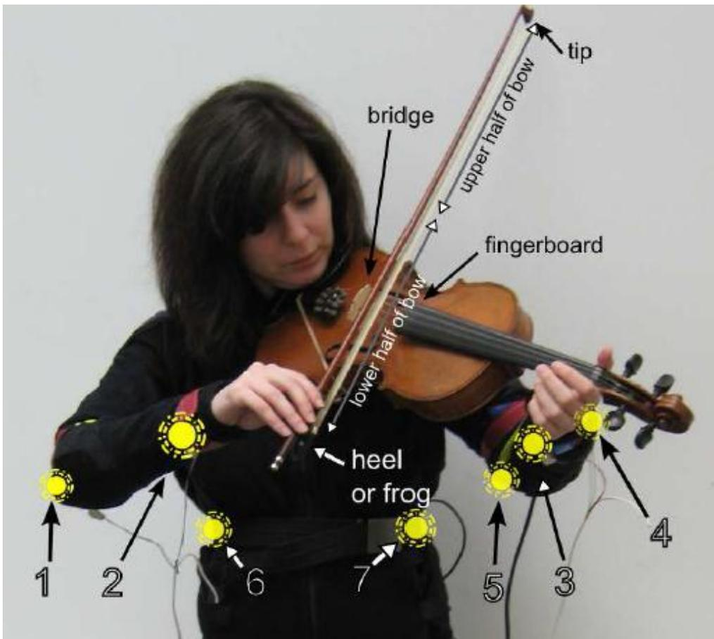
Figure 3-4: The MusicJacket (1 move bow hand forward, 2 move bow hand back, 3 move violin left, 4 move violin right, 5, 6, 7 lift violin)
