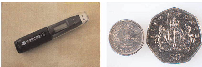
Figure 7. The integrated temperature and RH sensors used at Cottown (left) and Flatfield (right)
