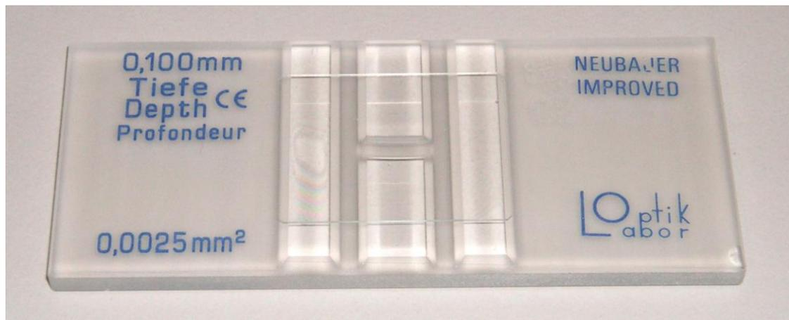
Figure 49- Neubauer improved counting chamber (from: Wikimedia commons).
