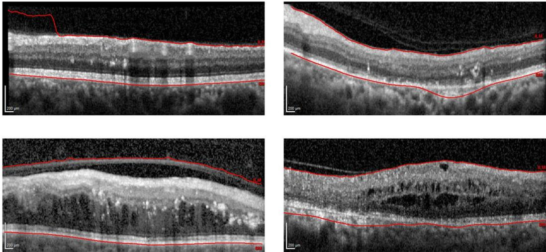
Figure 24 – Examples of boundary detection error. Top and bottom left: misplacement of ILM boundary. Top and bottom right – misplacement of BM boundary.
