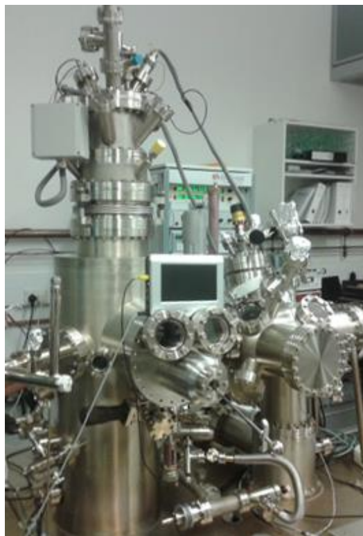
Figure 3.1 The LT STM used in this work consisting of three main parts; the vacuum system (only the LT STM chamber and the Preparation chamber can be seen in this figure), the electronic controller instrument (stored on the shelf behind the vacuum system), and the controlling computer (adjacent to the electronic controllers but cannot be seen in the photo).
