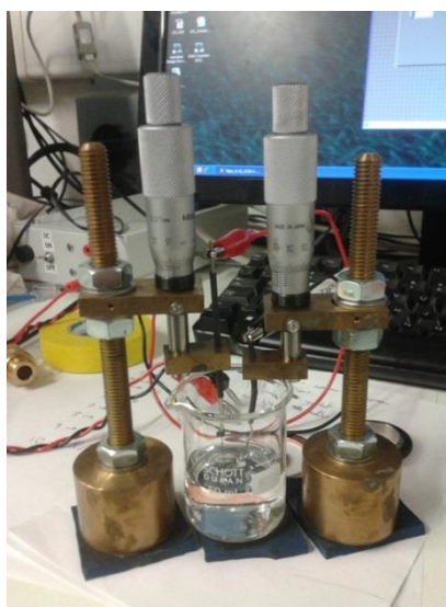
Figure 3.3 Instruments used for the tip-etching process. The beaker contains KOH solution with a stainless steel ring and a tungsten wire suspended from the micrometres, immersed into the solution and connected via a power supply.
