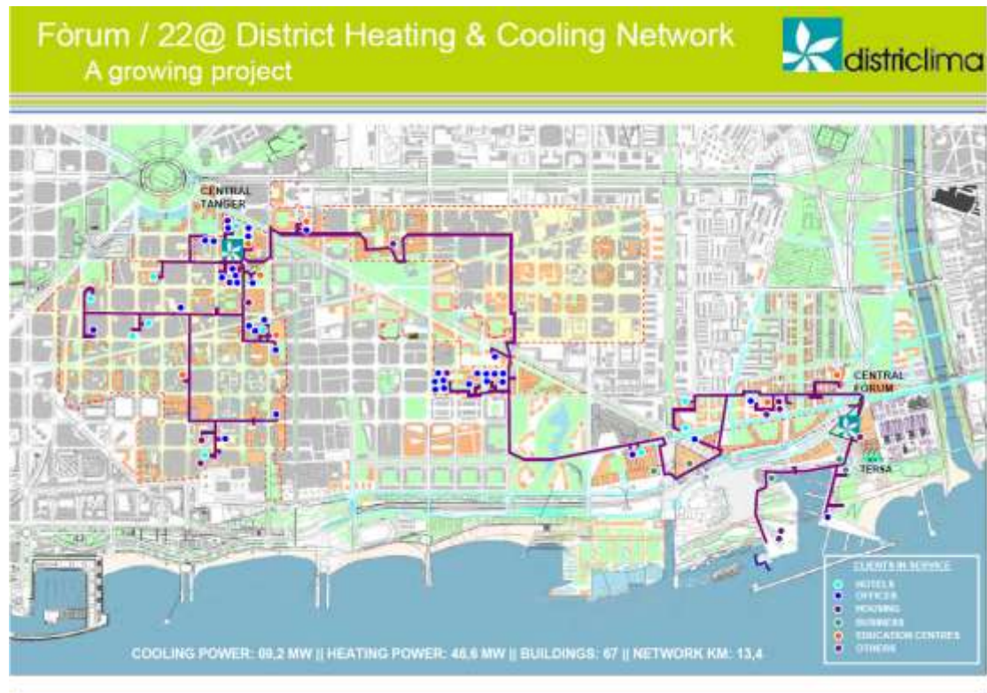
Figure 9: 22@ Districlima district heating and cooling system in 2012 (Districlima, 2012)
