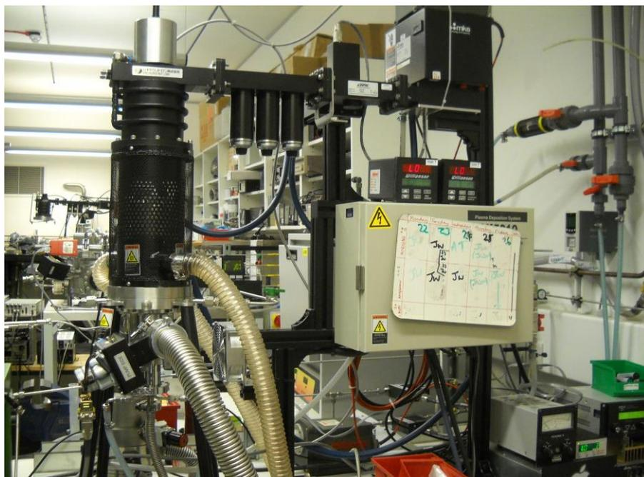
**Figure 3.11 Seki technotron PECVD setup**
