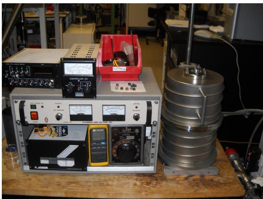
**Figure 3.12 High temperature nanodiamond hydrogen termination setup**
