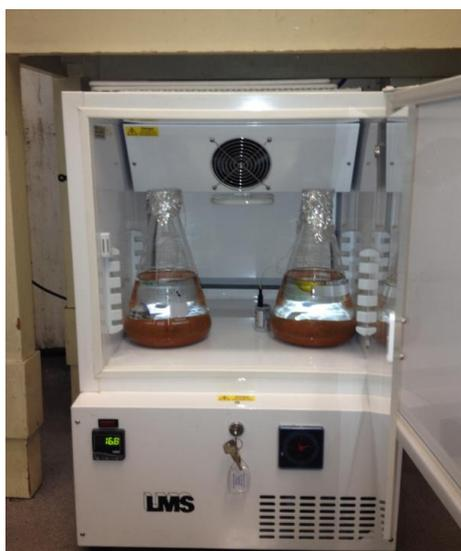
Figure 4-1: Erlenmeyer flasks located inside an isothermal cabinet (NHM, London).
