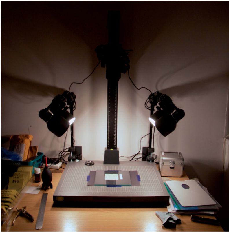
Fig. 4 Imaging set up for colour reflective imaging. The camera is locked facing vertically downwards. The sample is placed on the copystand over a piece of black card under a sheet of anti-reflective glass. The process of acquiring the images involved manually exchanging each filter in front of the camera lens, causing small movements of the camera each time (which meant the resulting images required further image registration, see Giacometti, 2013 )
