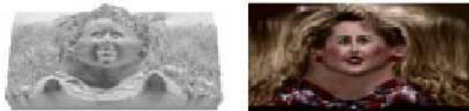
Figure 2.1 - Range data (left) and texture map (right) obtained with a Cyberware™ laser scanner
