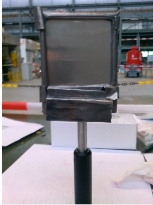
Figure 4.6: A photograph of the aluminium target in its holder with lead shielding covering the plastic holder.
