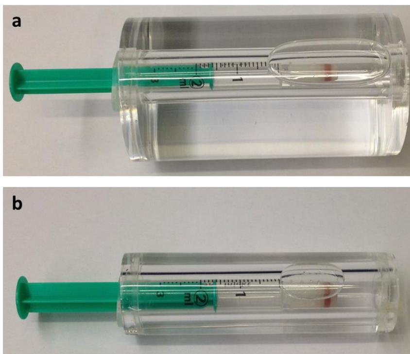
**Figure 13.** Quantification phantoms used for rat (a) and mouse apertures (b) on the SPECT/CT scanner.
