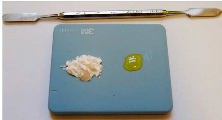
Figure 2-2: Filler powder and monomers mix on a rubber mixing pad before mixing.
