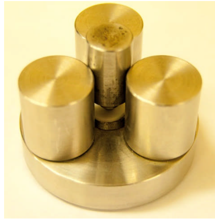
Figure 2-11: Ball-on-ring jig utilized for biaxial test method.
