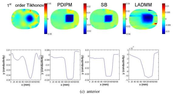
Figure 8. Reconstruction of the three perturbation positions in the head-shaped tank for each algorithm: 2D slice at z=7 cm and profile at z=0 cm of (a) posterior perturbation, (b) middle perturbation, (c) anterior perturbation
