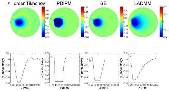
Figure 5. 2D slice at z=5 cm and profile plots at y=0 cm of the four algorithms for the cylindrical tank experiment
