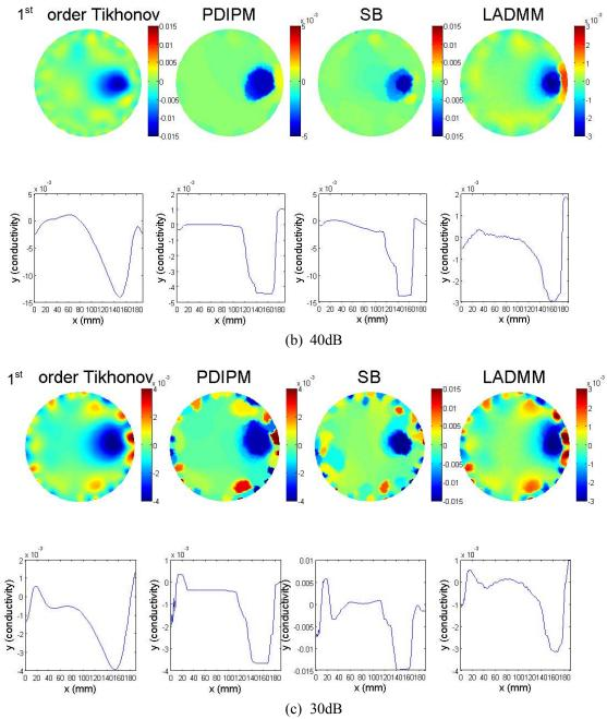
**Figure 2.** Illustration of the noise performance of the algorithms: 2D slice at z=5 cm and profile at y 0 cm of (a) 60 dB SNR, (b) 40 dB SNR, (c) 30 dB SNR
