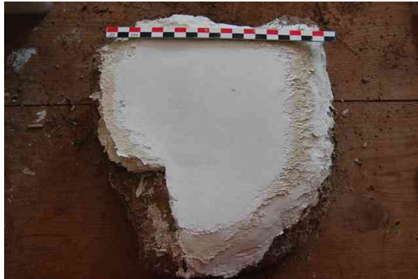
Fig.147 Marl plaster layer after burnishing with hands during application.
