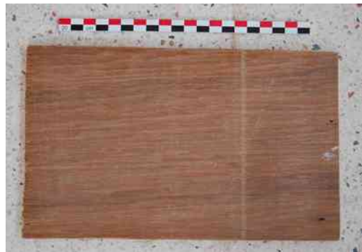
Fig.135 The wooden backing boards for the experimental plaster application.
