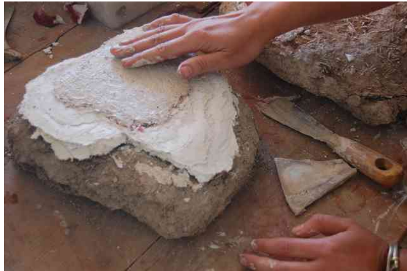
Fig.140 Application of marl plaster after thinning out with water.
