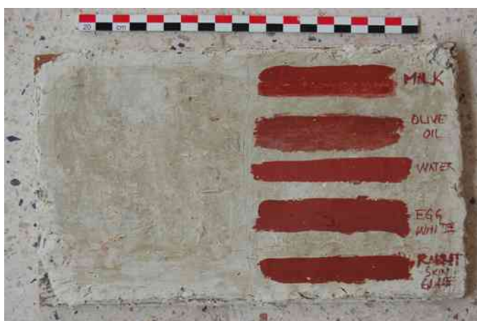
Fig.154a Painting experiments on dry marl plaster (burnished leather-hard) with six binders tested with red ochre pigment.
