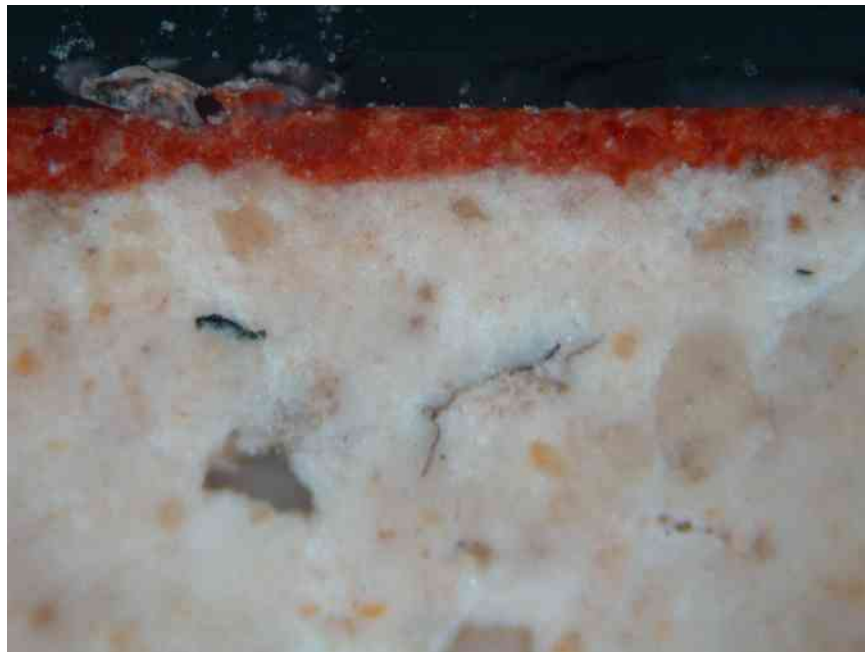
Fig.96 A cross section image of pigment layer by RLM, CH99/South/U.4844/S11, x400.
