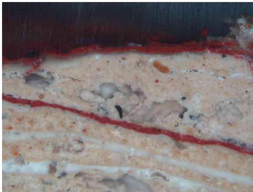
Fig.94 A RLM image of pigment layers, CH08/4040/U.16695/S1, x400.
