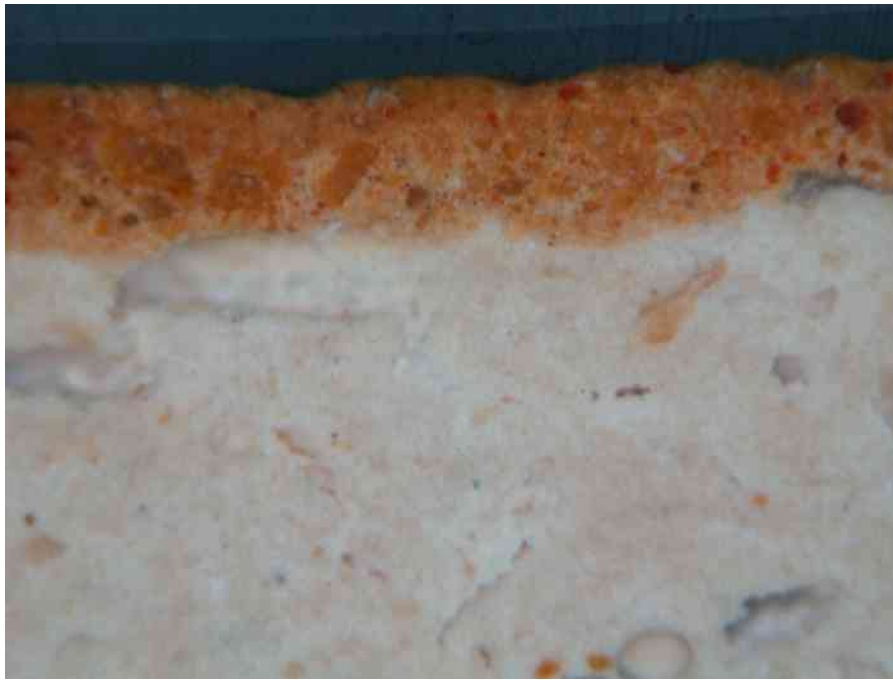
Fig.97 A cross section image of pigment layer by RLM, CH99/South/U.4709/S2, x400.
