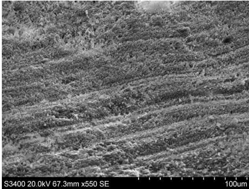
Fig.100b CH06/4040/U.13669/S2. SEM image of the same sample above at a higher magnification, showing details of sharp striations going in the same directions.
