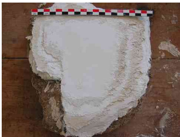
Fig.156 A thin layer of marl plaster burnished during application.
