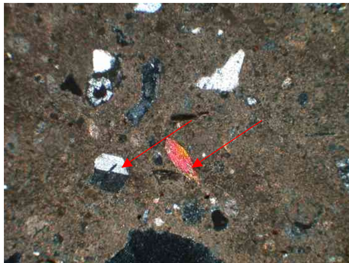
Fig.44 Feldspar and hornblende inclusions in Type 1 plaster, thin section image by PLM, CH96/North/U.1309/X1,2, x100.
