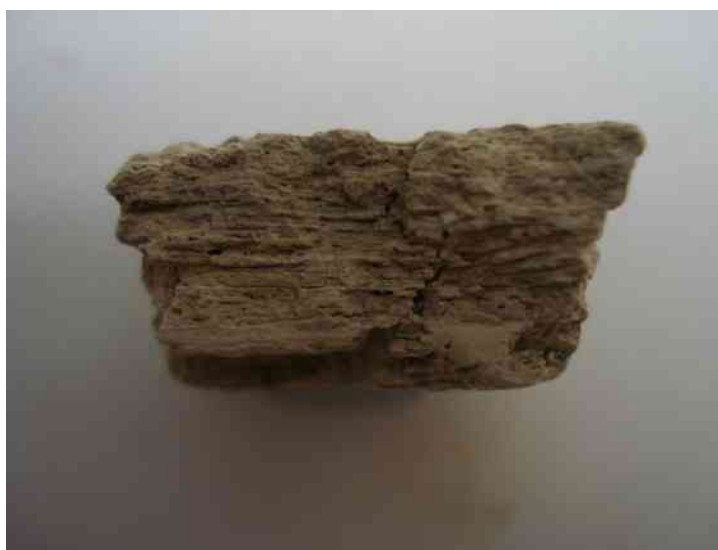
Fig.35 A multi layered plaster with white and pale brown layers, CH01/Bach/U.8203/S5.
