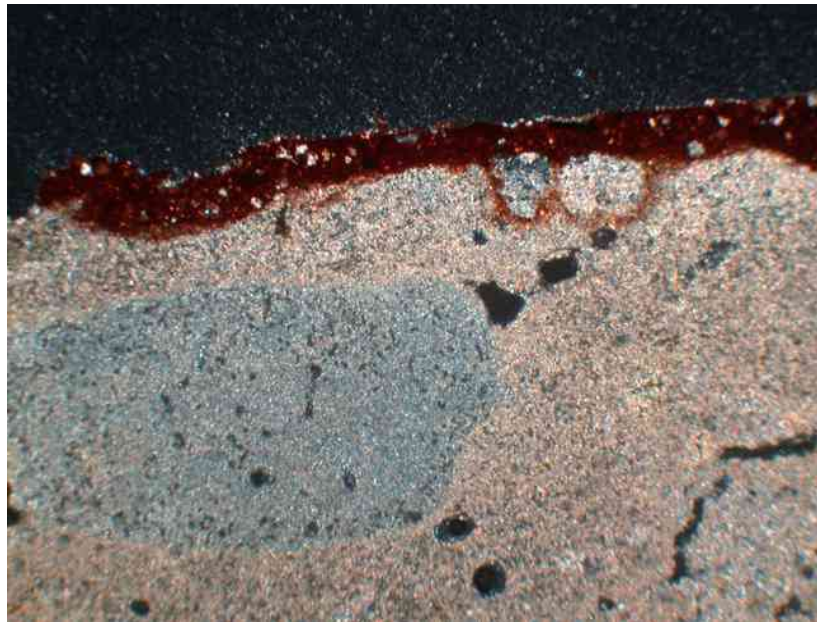
Fig.59 A thin section image of a Type 5 plaster by PLM, CH99/South/U.4629/S1 showing the single layered fine plaster with the red pigment layer above, x400.
