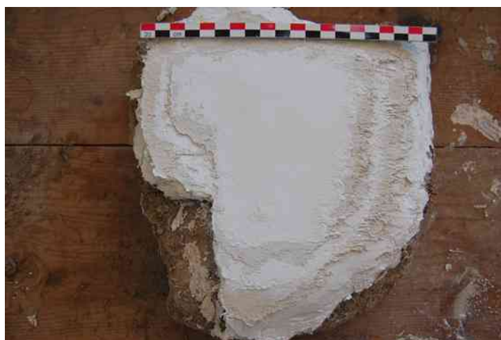
Fig.149 Marl plaster layer after burnishing, ready for painting.
