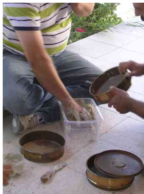
Fig.139 Mustafa and İbrahim mixing the sieved straw into marl.
