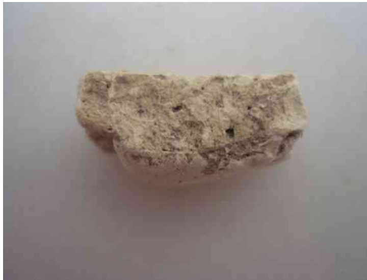
Fig.36 A single layered plaster with harder texture, CH99/South/U.5325/S6.
