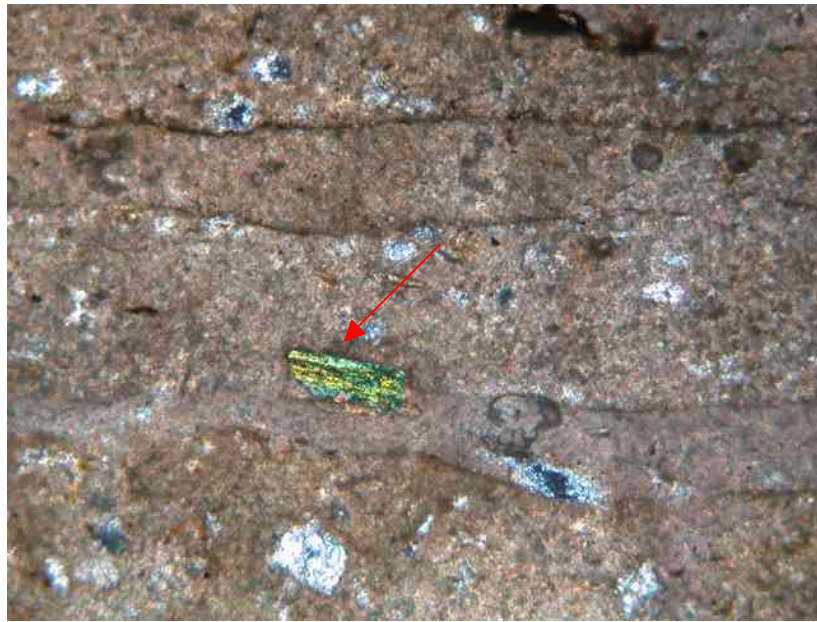
Fig.50 A thin section image of Type 2 plaster by PLM, CH01/Bach/U.8226/S3 with green hornblende inclusion, x400.
