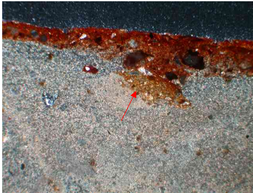
Fig.61 A thin section image of a Type 5 plaster by PLM, CH99/South/U.5273/S2 showing an evidence of recycled painted plaster fragment being used as added inclusions, x100.
