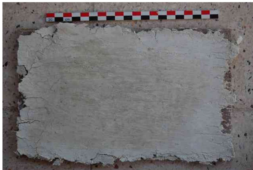
Fig.148 Marl plaster layer after burnishing when leather-hard.
