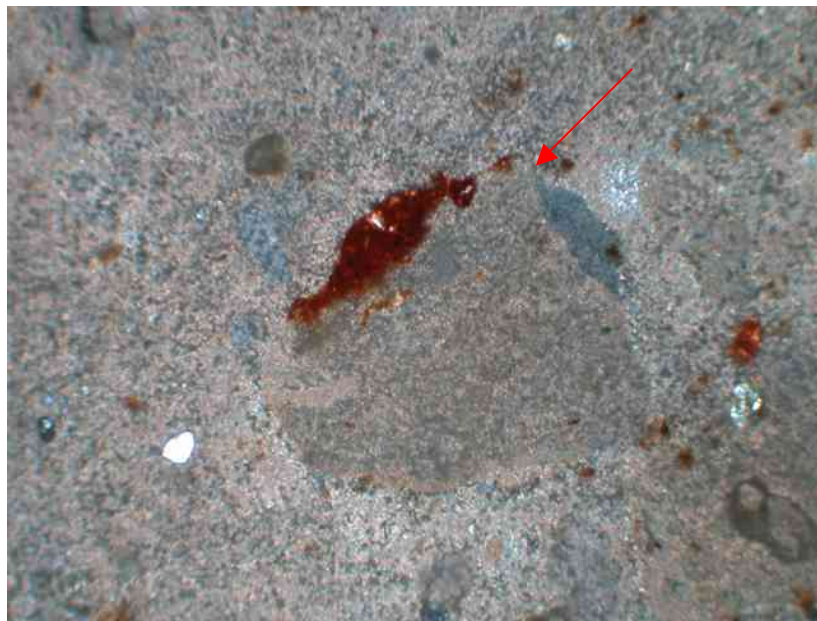
Fig.60 A thin section image of a Type 5 plaster by PLM, CH99/South/U.5273/S2 showing an evidence of recycled painted plaster fragment being used as added inclusions, x400.
