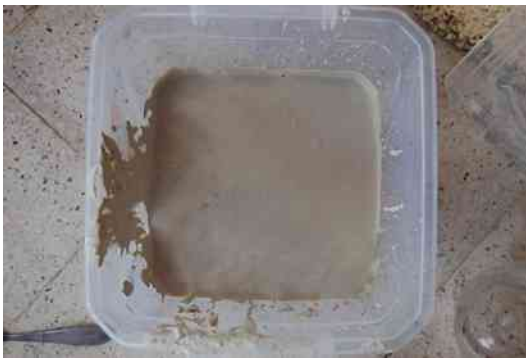
Fig.134 Soaking the marl lumps in water.
