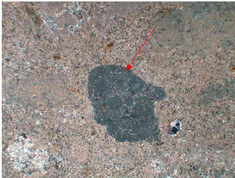
Fig.66 A thin section image of a Type 5 plaster by PLM, CH99/South/U.5294/S6 showing an andesite inclusion, x400.
