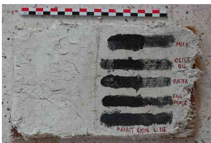
Fig.154b Painting experiments on dry marl plaster (burnished leather-hard) with six binders tested with carbon black pigment.
