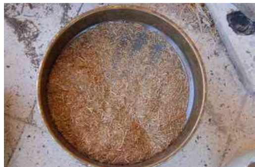
Fig.136 Finely sieved straws to add into marl plaster.
