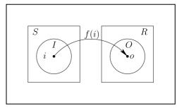
Fig. 1. Stimulus and observations: *S* is anything that can change the observable behavior of the SUT *f*; *R* is anything that can be observed about the system's behavior; *I* includes *f*'s explicit inputs; *O* is its explicit outputs; everything not in  $S \cup R$  neither affects nor is affected by *f*.
