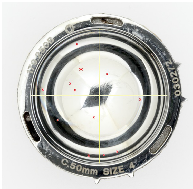
Fig 5 Location of primary wear scars. An image of a metal cup on which each of the 13 wear scars is superimposed, according to which quadrant the wear scar was positioned
