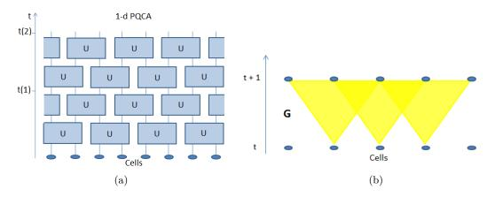
Figure 3.2: (a) Sketch of the 1-dimensional  $\frac{1}{2}$ -nearest neighbor QCA evolution in time. Wires are cells, time flows upwards. One iteration of the automaton corresponds to the application of two layers of local two-qubit unitaries. (b) The light cone of a QCA.
