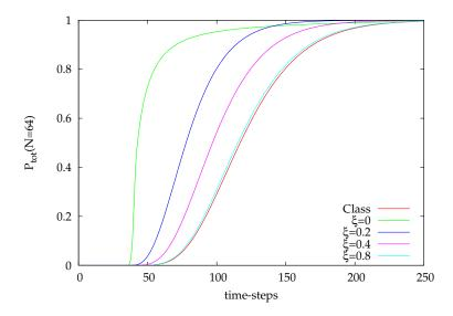
Figure 3.4: Integrated probability of absorption through an open chain with N = 64, p = 0.7, q = 0.5,  $\varphi_1 + \varphi_2 = \pi$  (the probability only depends on the sum  $\varphi_1 + \varphi_2$ ) and various values of  $\xi$ , from classical ( $\xi = 1$ , denoted by "Class") to most quantum ( $\xi = 0$ ).
