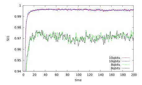
Figure 5.1: Mean Von Neumann reduced entropy  $\langle S(\rho_i(t)) \rangle$  on one site of a 1-dimensional PQCA of 8 and 10 qubits. Each line refers to an average over an ensemble of 250 different evolutions, each of which given by a different local unitary drawn at random according to the Haar measure. Even for such small size systems the reduced entropy is very close to the maximum value.
