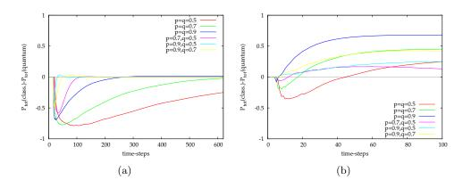
Figure 3.6: Difference between most classical ( $\xi = 1$ ) and most quantum ( $\xi = 0$ ) integrated probabilities of absorption through a ring with  $\varphi_1 = \varphi_2 = 0$ , various values of p and q, and N = 64 (a) and N = 18 (b).
