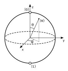
Figure 1.1: Bloch sphere representation of a qubit.
