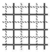
Figure 3.1: A schematization of the so-called Margolus partitioning scheme in s = 2 dimensions. Operations are alternatingly applied to the solid and to the dashed partitioning into  $2 \times 2$  squares. Here cells are represented as squared, but their actual shape can be different, as it only serves to label localized quantum systems.
