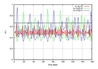
Figure 4.1: Average fidelity  $\langle F(t) \rangle$  over a sample of 1000 evolutions starting from initial states drawn at random from the Haar measure, for p = q = 0.5 and three different choices of  $(\varphi_1, \varphi_2)$  on a linear chain of N = 8 qubits. No noise applied. The straight horizontal line at F = 2/3 shows the highest fidelity for classical transmission of a quantum state.
