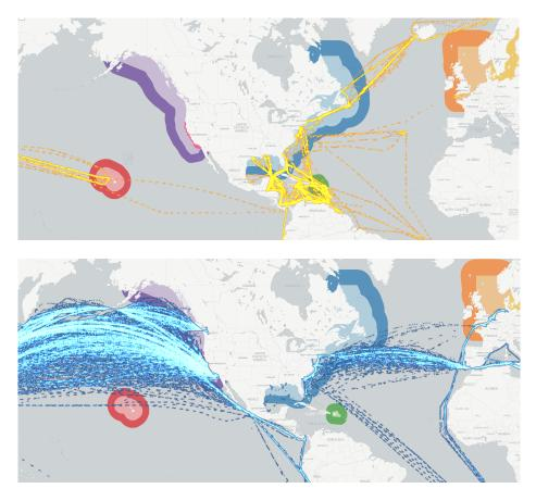
Figure 3. Route network by container vessels that enter the North American ECA of size bin 1 (top) and size bin 6 (bottom).
