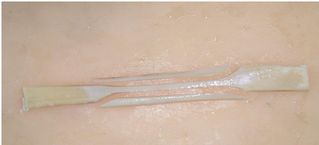
Figure 4.3: DCB strip cut into dog bone shape prior to mechanical testing
