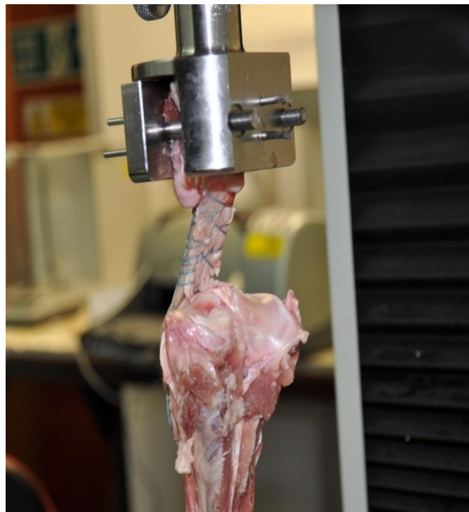
Figure 3.4: Mechanical testing of the cadaveric patellar tendon repair models
