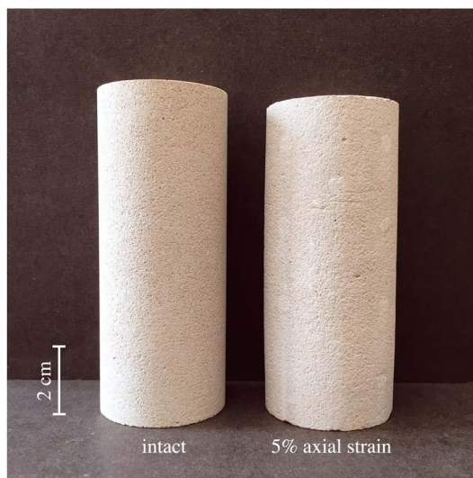
Figure 1. Photograph of an intact sample and a sample deformed up to 5% axial strain at P_{\text{eff}} = 50 MPa.
