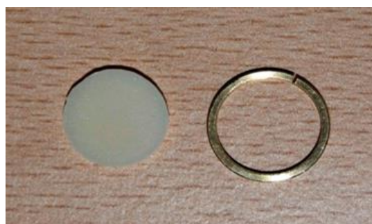
Figure 5-2 : Light cured dental composite disc (10 × 1mm thickness) after removed from metal ring.
