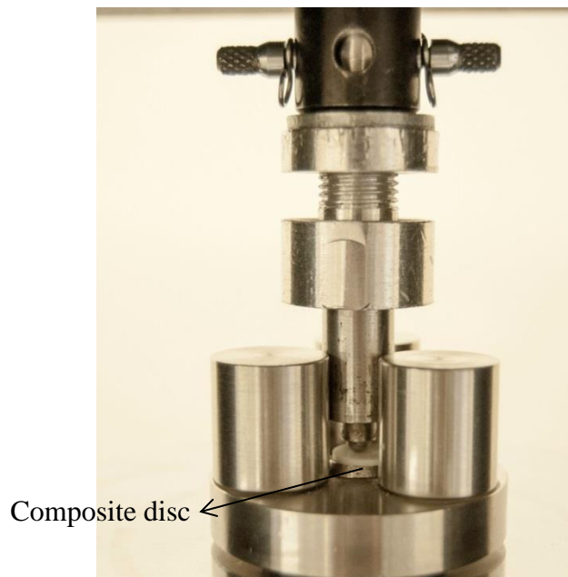
Figure 5-7: BFS jig with ‘ball on ring’ jig.
