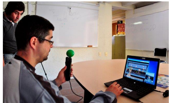
Fig. 1. The Gesture Therapy platform. One of the researchers is illustrating the use of it. The gripper, hold with the left hand here, serves to control an avatar on the virtual scenario. 3D location of the hand and gripping pressure are sensed and send to the computer for further processing.
