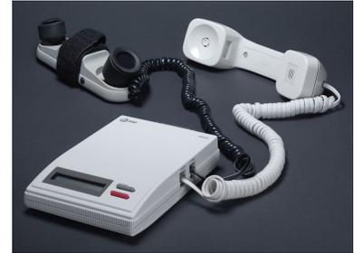
Figure 3: The AT&T TSD-3600E: one voice encryption product based around the Clipper chip. (Photo: Matt Blaze)
