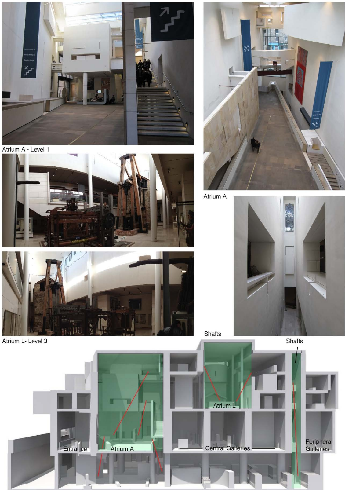
Figure 3. Views and three-dimensional section through the atria, the shafts and galleries in the Museum of Scotland.
