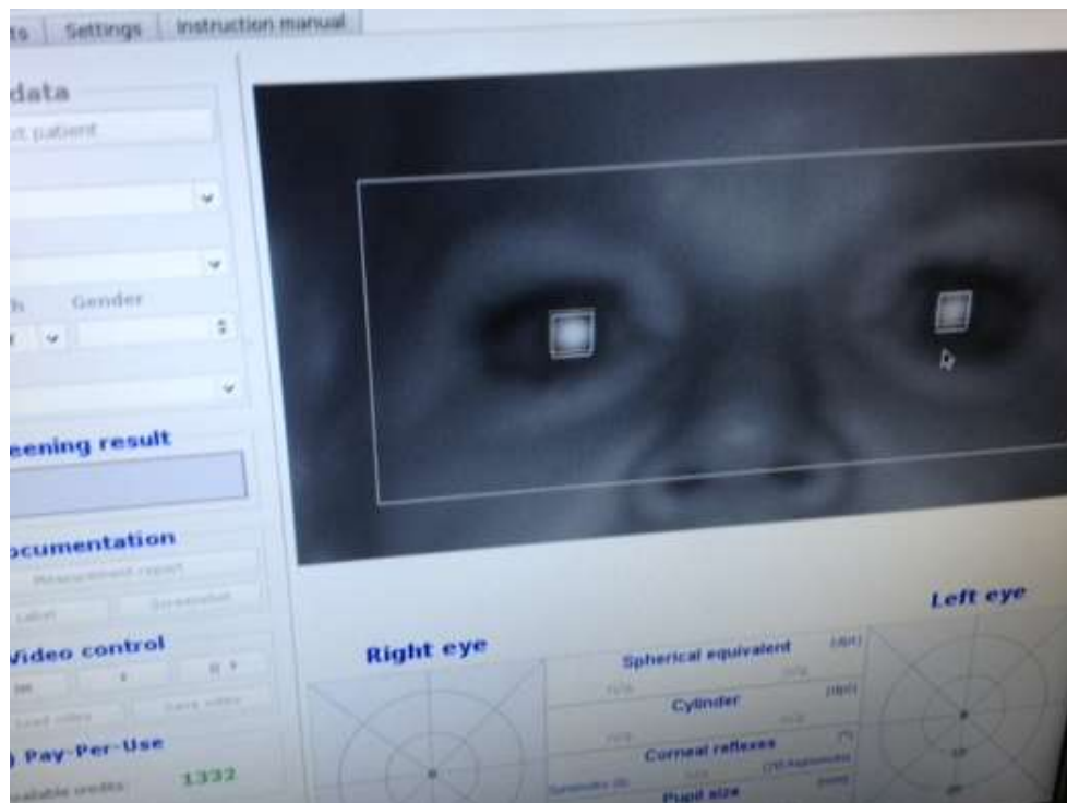
Figure 11. PlusoptiX measurement process - white squares over pupils
