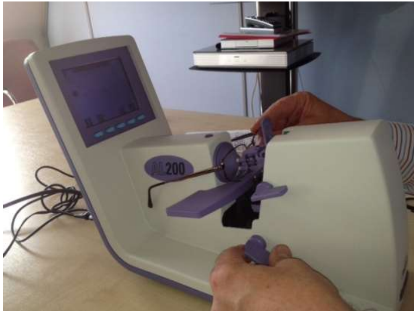
Figure 21. Focimeter with glasses in place to measure the right lens
