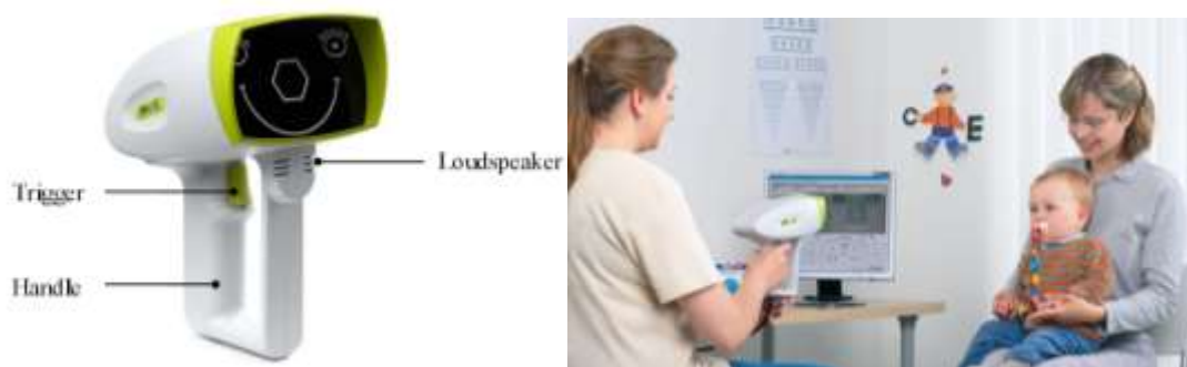
Figure 2. PlusoptiX autorefractor device head
