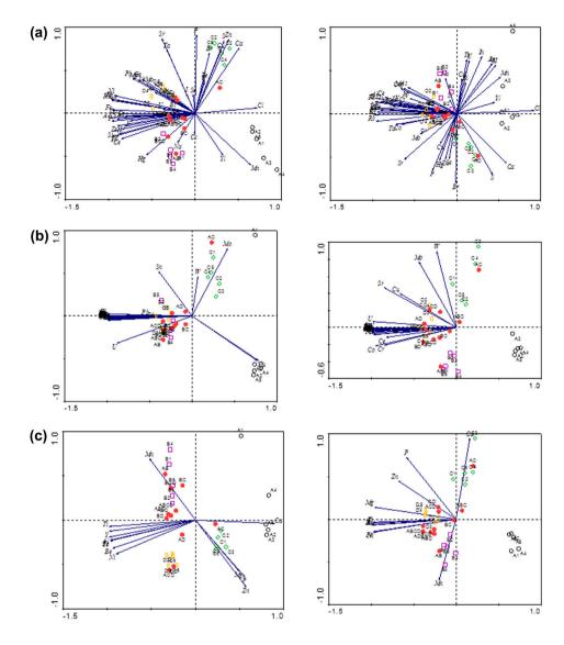
Figure 4. PCA graphs illustrating the significant elements found for single source and mixed source samples via a) XRF, b) ICP-MS and c) ICP-AES in March (left) and May (right). (Site A - black outlined circle, Site B - purple square, Site C - green diamond, site D - yellow rectangle, mixed sites - red filled circle).
