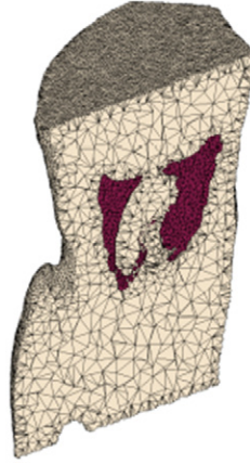
Figure 3. Mesh cross section. The mesh is finer within the region of interest, i.e. the lungs.
