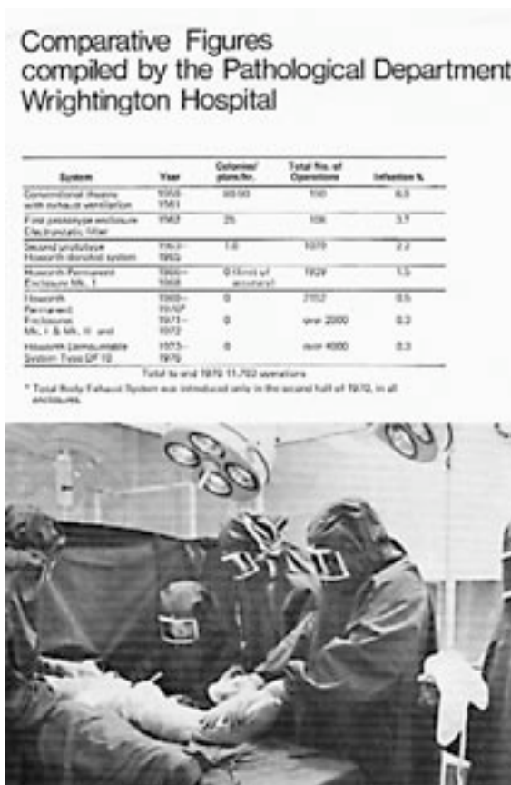
Figure 24: Howarth publicity literature on the influence of the clean-air enclosure (the inside of the enclosure is shown here) and the surgeons' full-body exhaust suit, c. 1976.
