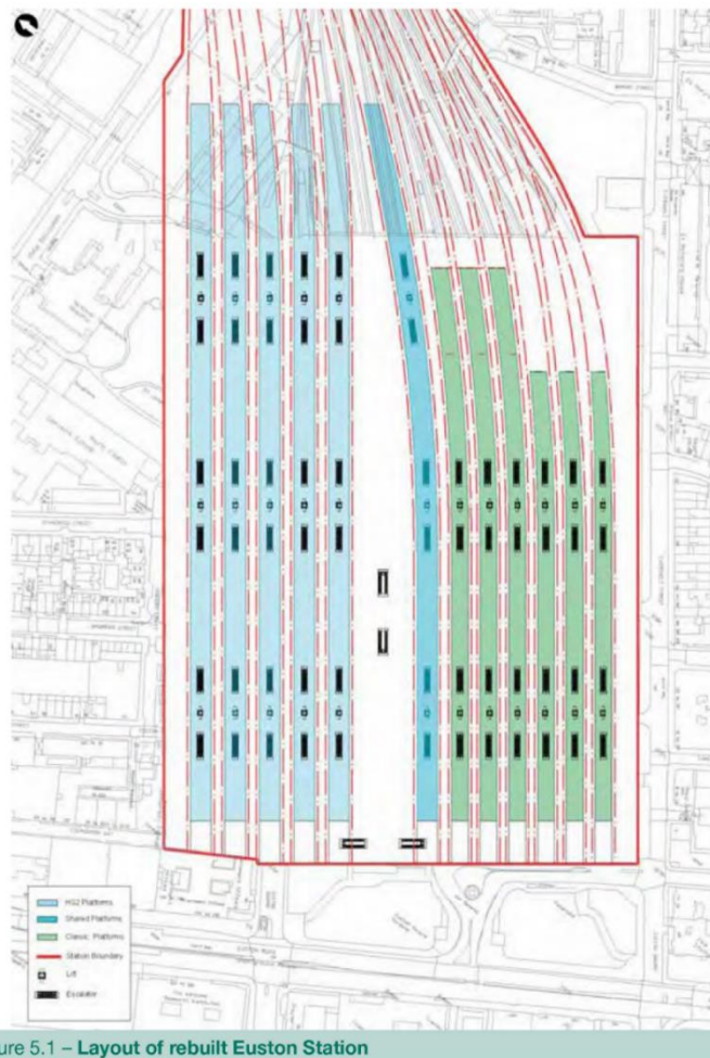
Figure 5.14: Platform requirement at Euston, HS2 Platforms in blue (HS2Ltd/DfT, 2011a).
