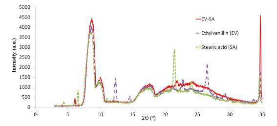
Figure 3: Comparison of the XRD curves of pure EV, pure SA and EV with SA nanoparticles, 4 wt% SA nanoparticles containing 1.6 wt% EV, prepared at a flow rate  $15 \mu \text{lmin}^{-1}$  and applied voltage 14.5 kV. All curves were recorded with the same temperature calibration. On the Intensity axis, a.u. indicates arbitrary units.
