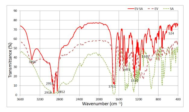
Figure 4: FT-IR spectra of pure EV, pure SA and EV with SA nanoparticles, 4 wt% SA nanoparticles containing 1.6 wt% EV, prepared at flow rate  $15 \,\mu \text{l min}^{-1}$  and applied voltage  $14.5 \,\text{kV}$ . The nanoparticle spectra show peaks that are characteristic of both pure EV and pure SA.
