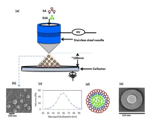
Figure 1: Schematic illustration; (a) EHD set-up. (b) SEM image of 4 wt% stearic acid lipid nanoparticles encapsulating 1.6 wt% EV in their structure generated at an applied voltage of 14.5 kV and flow rate of  $15 \,\mu \text{l}\,\text{min}^{-1}$ . (c) Size distributions of nanoparticles containing EV. (d and e) schematic and corresponding TEM image of a nanoparticle. Average size is  $65 \pm 6 \text{ nm}$ . Scale bar 100 nm.
