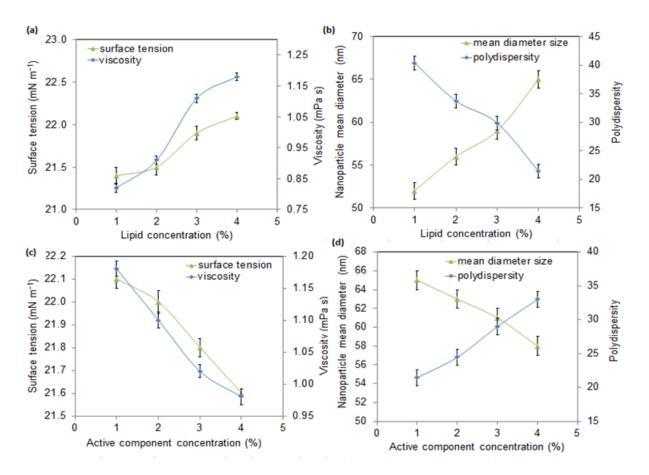
Figure 2: (a) Effect of lipid concentration, surface tension and viscosity of solution, (b) mean diameter and polydispersity of nanoparticles prepared at different stearic acid lipid concentrations. Effect of EV weight concentration (wt%) on 4 wt% of lipid solution on: (c) surface tension, and viscosity, (d) mean diameter and polydispersity.  $N \simeq 300$  nanoparticles.
