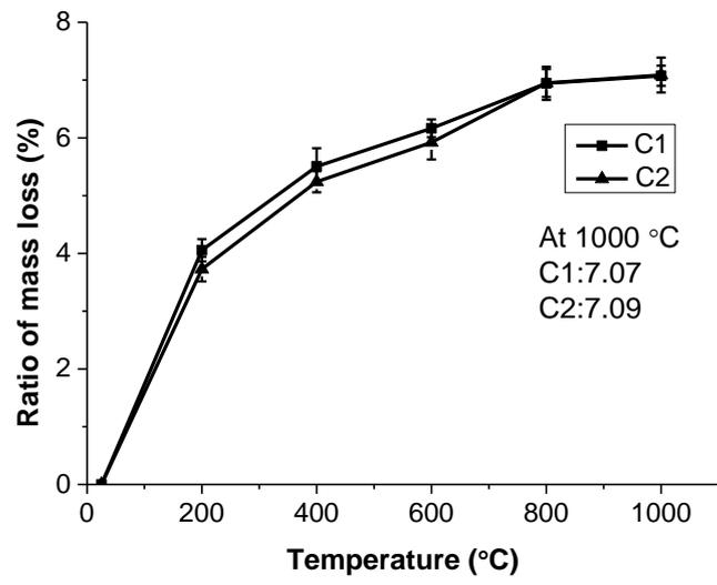
**Fig. 7.** Ratio of mass loss of FSCs at different temperatures
