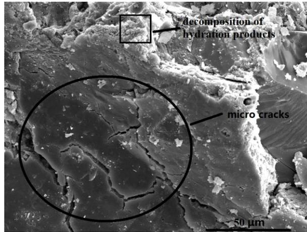
**Fig. 9.** SEM image of FSC with PP fibers after heating to 600 °C
