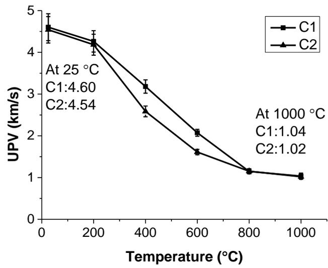
**Fig. 5.** The UPV of FSCs before and after exposure to high temperatures
