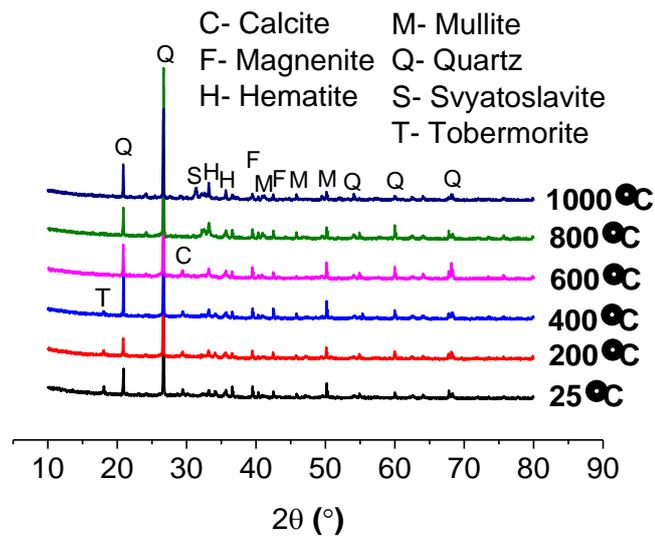
**Fig. 10.** XRD patterns of FSC with PP fibers before and after high temperatures exposure. Phases identified: calcite,  $\text{CaCO}_3$ ; magnetite,  $\text{Fe}_3\text{O}_4$ ; hematite,  $\text{Fe}_2\text{O}_3$ ; mullite,  $\text{Al}_{4.8}\text{Si}_{1.2}\text{O}_{9.5}$ ; quartz,  $\text{SiO}_2$ ; svyatoslavite,  $\text{CaAl}_2\text{Si}_2\text{O}_8$ ; tobermorite,  $\text{Ca}_5(\text{HSi}_3\text{O}_9)_2 \cdot 2\text{H}_2\text{O}$ .
