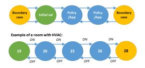
Figure 3: A state diagram models an HVAC maintaining the room temperature between 20 and 26°Celsius. The user also specifies an negative policy for temperature reaching 25°Celsius.
