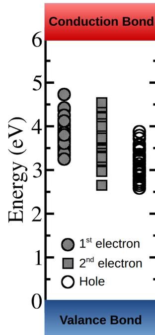
FIG. 2. Distribution of the KS levels for the electron and hole trapping in a-HfO<sub>2</sub> structures with 324 atoms. The energy scale from 0.0 to 6.0 eV corresponds to the a-HfO<sub>2</sub> band gap as calculated using the PBE0-TC-LRC functional.
