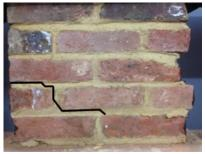
Figure 3: Failed masonry wallette showing location and extent of shear crack
