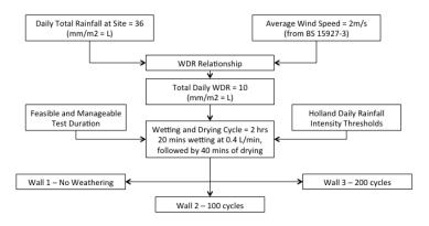
Figure 1: Route map demonstrating weathering sequence design process
