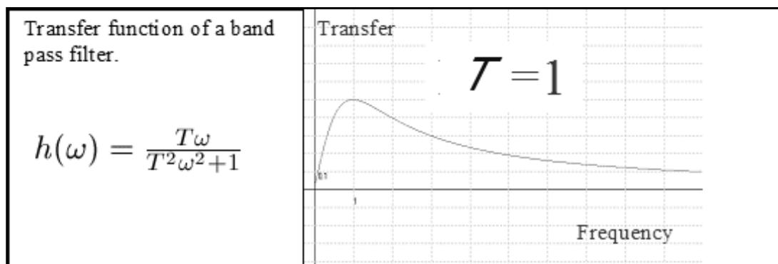
**Figure 2.7 :** *The band pass filter.*
