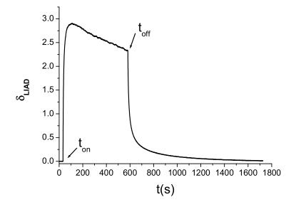
**Figure 2.** Typical example of an LIAD (Light Induced Atomic Desorption) signal: Rb relative vapor density variation as a function of time in a polydimethylsiloxane (PDMS) coated cell.  $t_{on}$  and  $t_{off}$  indicate the time when the desorption light ( $I_L = 17 \text{ mW/cm}^2$  at 514 nm) is turned on and off.
