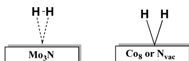
Scheme 1. Simplified Schematic Showing (a) Molecular and (b) Dissociative Adsorption of H 2 on Co 3 Mo 3 N Surfaces
