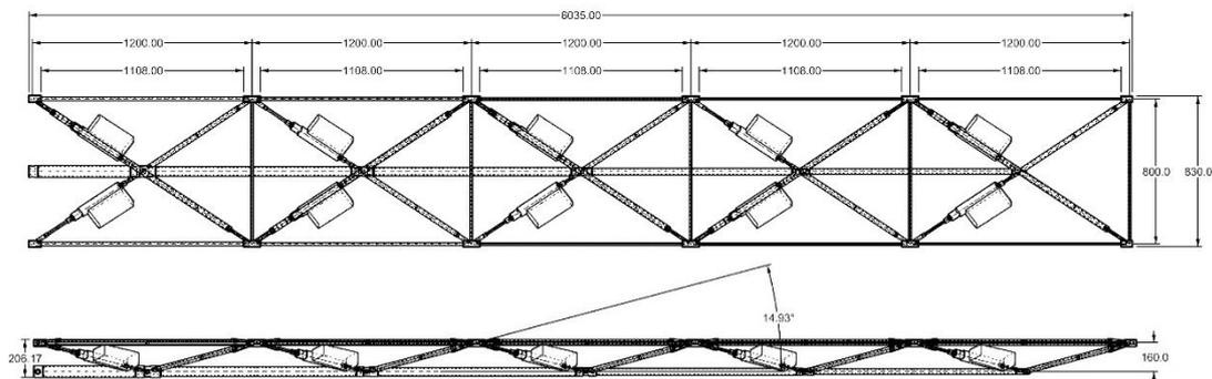
Figure 7: adaptive truss overall dimensions
