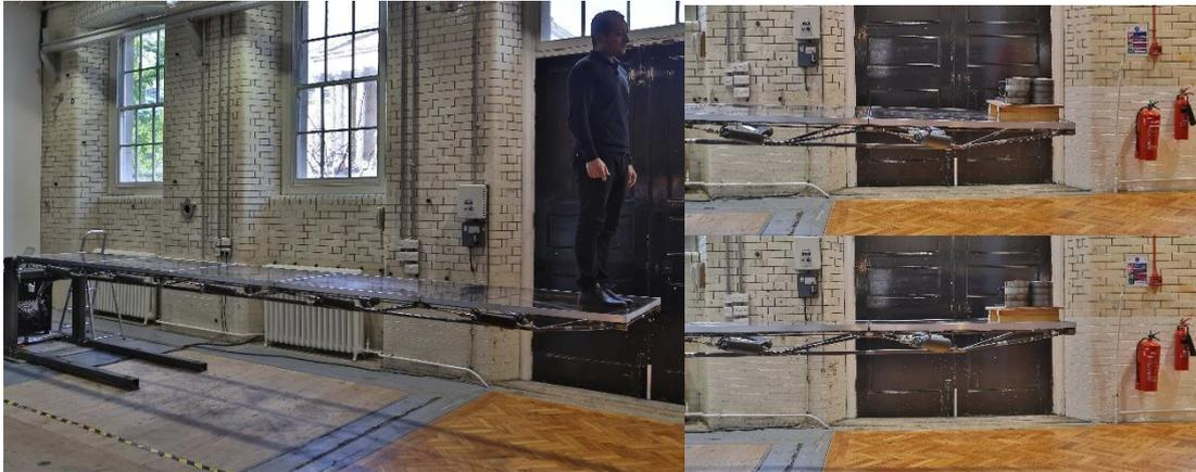
Figure 14: control person walking (left); 100kg no control (top right); 100kg controlled (bottom right) are recorded when a person walks on the deck (fig. 14). During the walk the actuators move subtly to continuously compensate for the moving load achieving a very stable control. Interestingly during control the movement of the structure are almost not perceivable to the observer and they become more noticeable when a load (weights or person trying to push the structure) is applied suddenly.
