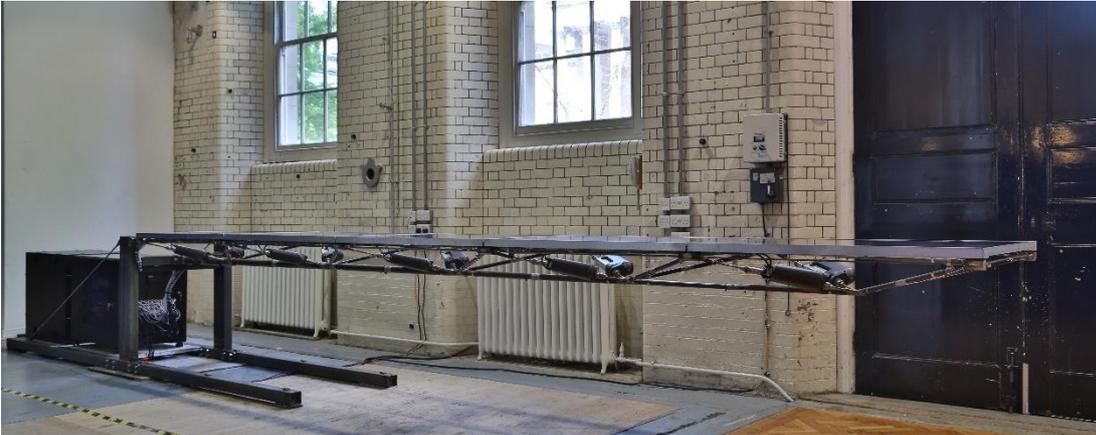
Figure 6: adaptive truss prototype, UCL structures laboratories
