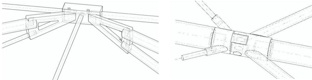
Figure 8: top chord node (left); bottom chord node (right);
