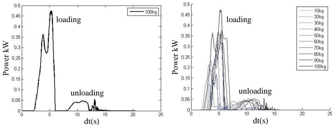
Figure 16: power measurement (current sensor)
