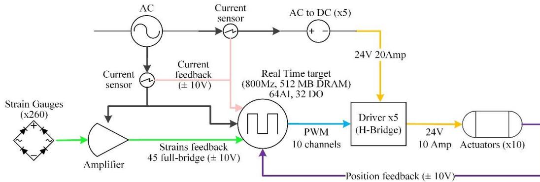
Figure 10: control hardware architecture
