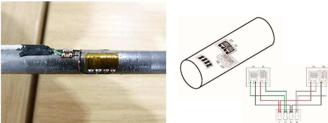
Figure 11: full bridge strain gauge sensor
