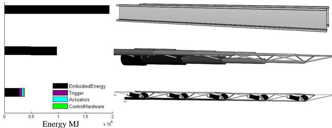
Figure 17: energy comparison (a) I-beams (b) optimised passive truss (c) adaptive truss
