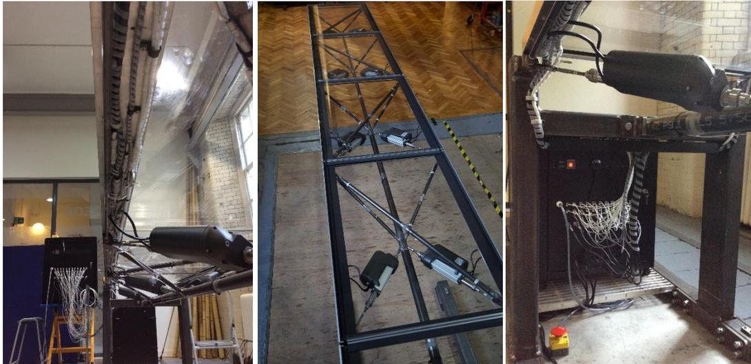
Figure 12: signal cables (left); actuators integrated (middle); actuator close up (left)
