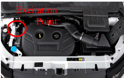
Figure 2 (a): The bonnet interior of a Range Rover Evoque, with the site at which the vehicle is excited with the impact hammer.
