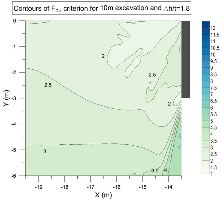
Figure 16. Contours of  $F_{D\sigma}$  for the 10m excavation case with  $\Delta h = 1.8t$
