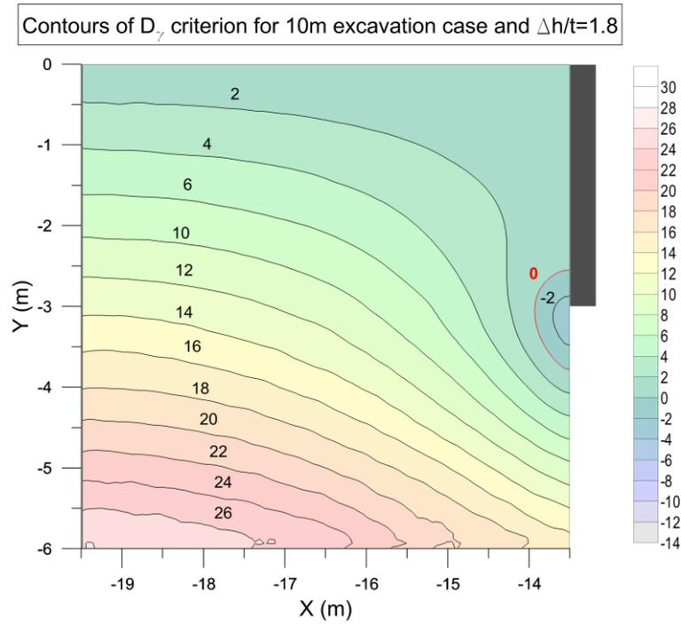
Figure 10. Contours of  $D_7$  for the 10m excavation case with  $\Delta h = 1.8t$
