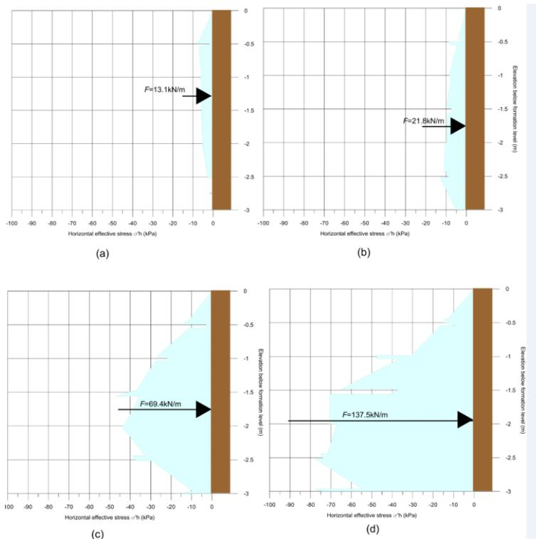
Figure 20. Horizontal effective stress distributions and resultant forces in front of the retaining wall for a) cofferdam with  $\tan\delta=0.5\tan\phi'$ , b) cofferdam with  $\delta=\phi'$ , c) 10m deep excavation with  $\tan\delta=0.5\tan\phi'$  and d) 10m deep excavation with  $\delta=\phi'$ .
