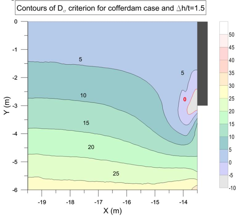
Figure 13. Contours of  $D_\sigma$  for the cofferdam case with  $\Delta h = 1.5t$
