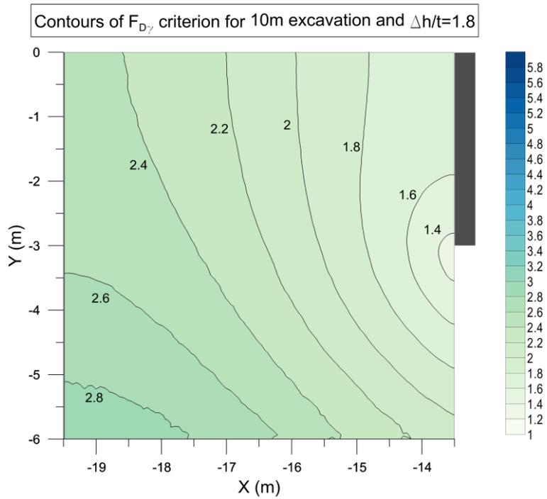
Figure 14. Contours of  $F_{D\gamma}$  for the 10m excavation case with  $\Delta h = 1.8t$
