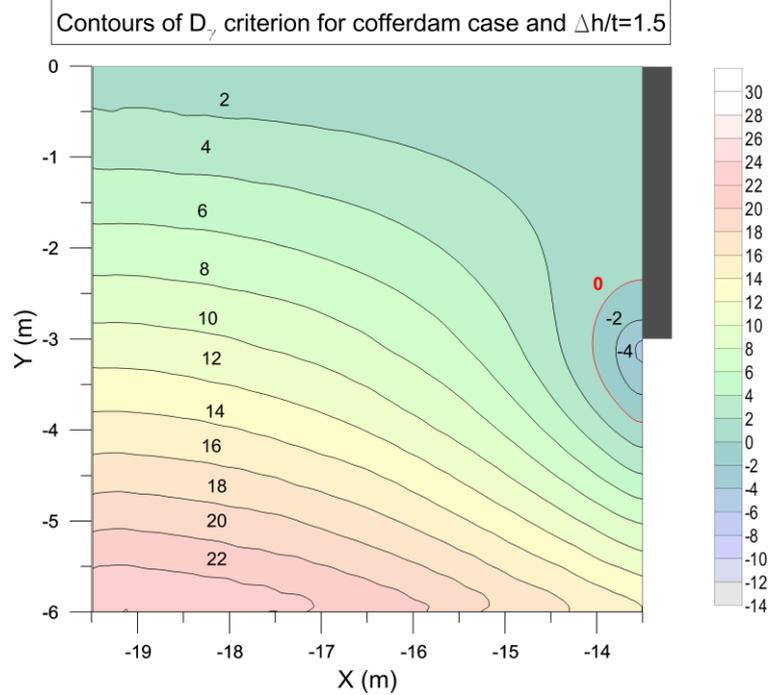
Figure 11. Contours of  $D_7$  for the cofferdam case with  $\Delta h = 1.5t$
