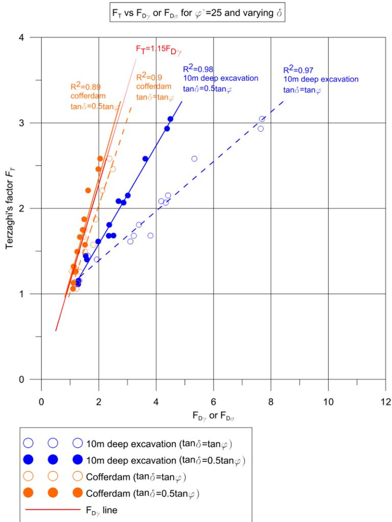
Figure 21. Relationship between the Terzaghi's factor  $F_T$  and the integration point approach factors  $F_{D\gamma}$  and  $F_{D\sigma}$  for  $\varphi'=25^\circ$  and varying soil/wall friction angle  $\delta$ .
