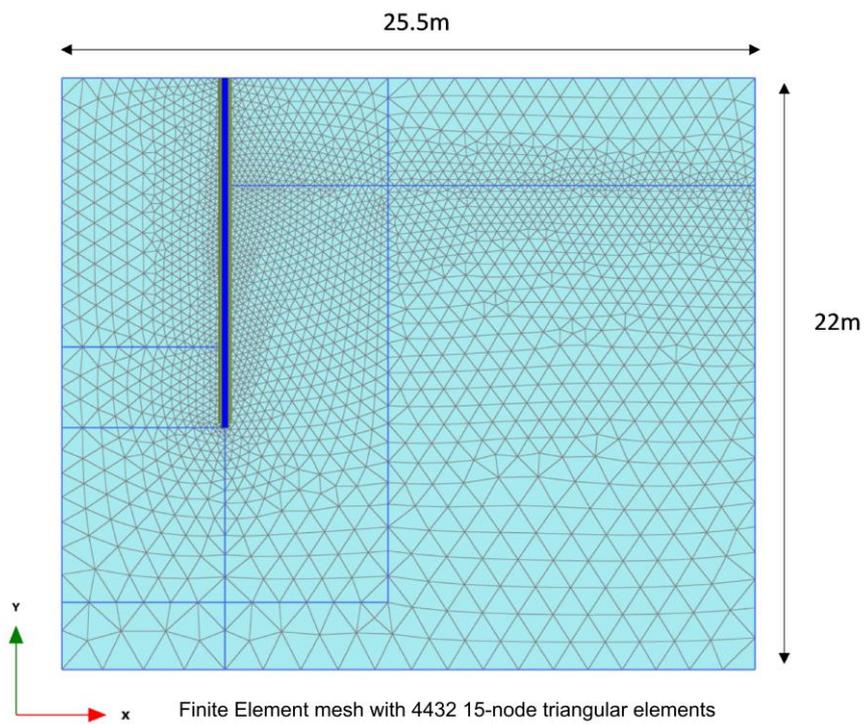
Figure 3. Finite Element mesh for the 10m deep excavation model
