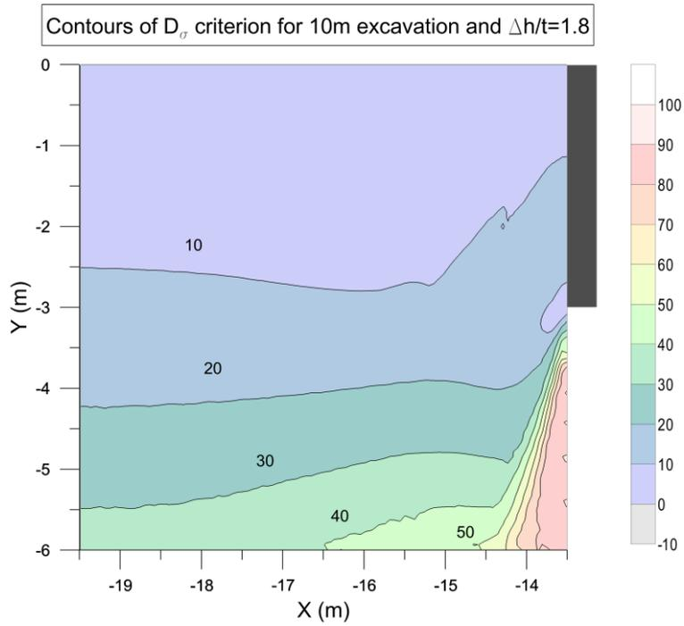
Figure 12. Contours of  $D_\sigma$  for the 10m excavation case with  $\Delta h = 1.8t$
