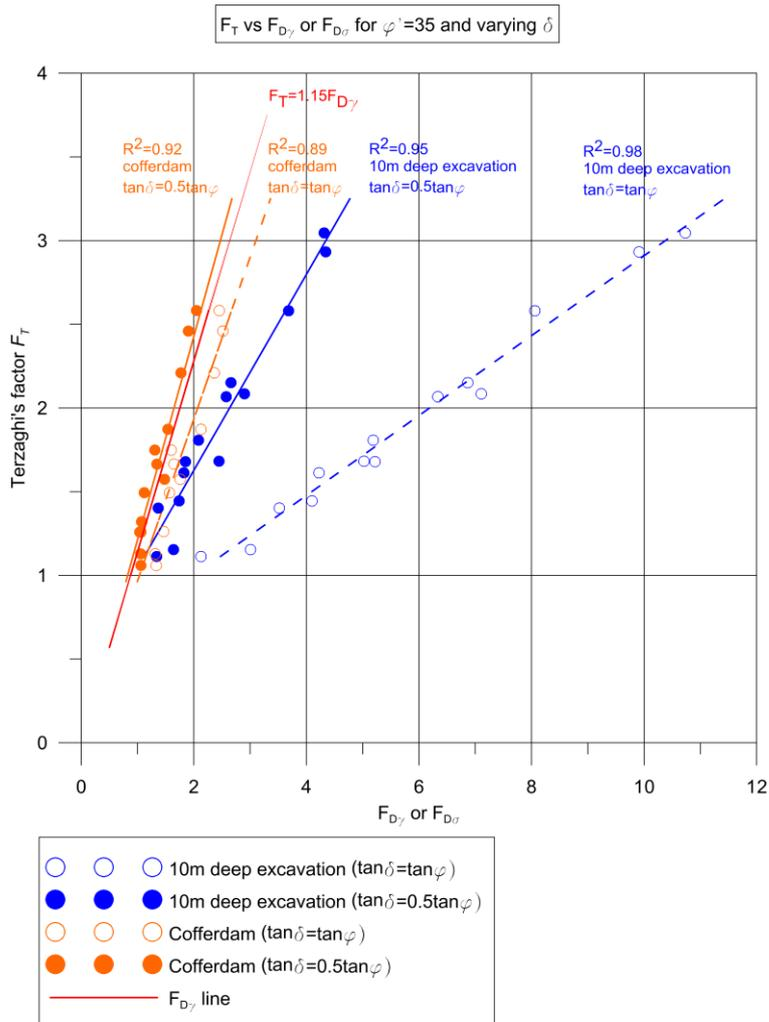
Figure 19. Relationship between the Terzaghi's factor  $F_T$  and the integration point approach factors  $F_{D\gamma}$  and  $F_{D\sigma}$  for  $\varphi'=35^\circ$  and varying soil/wall friction angle  $\delta$ .
