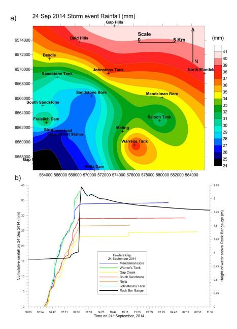
Fig. 8 a) Rainfall distributions over a 1-day event on 24 September 2014. b) Hyetographs and runoff measured at Fowlers Gap stream gauge (refer to Figure 1b and 1c).
