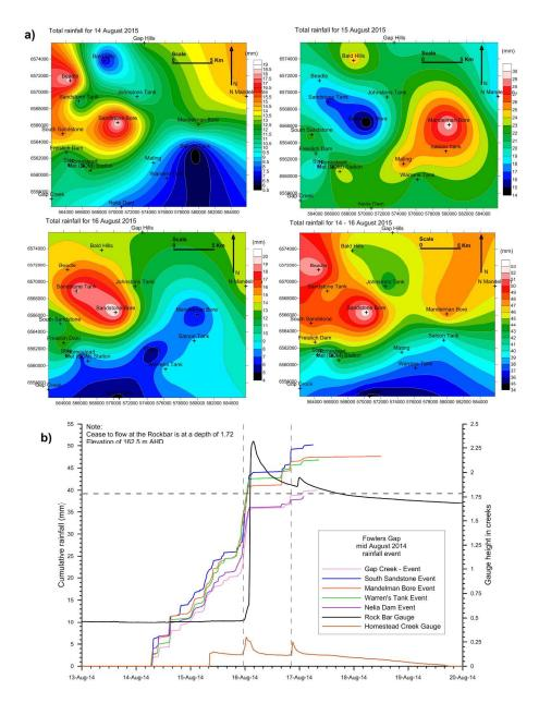
Fig. 7 a) Rainfall distributions over a 3-day event in August 2014. b) Hyetographs and run off at the Rock Bar and Homestead Creek stream gauges (refer to Figure 1b and 1c). 200x265mm (300 x 300 DPI)
