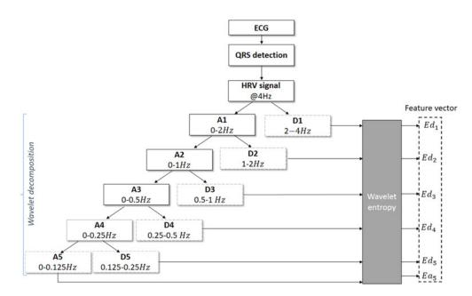
Fig. 3. Flowchart of the feature extraction algorithm.
