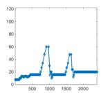
Fig. 3 OSSPSauto experiment. Left plot shows the cosine of the angle between the 2 subset updates at each step in the algorithm. Right plot shows the selected number of views used per update. Horizontal axis in both plots is the cumulative number of views used.
