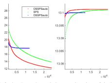
Fig. 4. Left plot shows the evolution over iterations of the Mean Square Error (MSE) between the reconstructed image with OSEM and the true image. Right shows the penalised log-likelihood. The horizontal axis in both plots is the cumulative number of views used.
