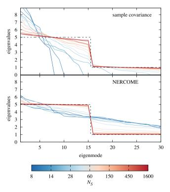
**Figure 1.** Spectrum of eigenvalues of an  $N_{\rm D}=30$ -dimensional covariance estimate for the toy example of uncorrelated data with standard errors of 1 and 5 for 50 per cent of the data set, respectively (see black dashed line). Coloured curves result for different numbers of realizations of the data,  $N_{\rm S}$ . Top panel: sample covariance estimates. Bottom panel: NERCOME estimates.
